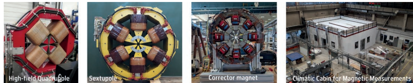
Figure 6 PETRA IV high-field quadrupole (PQA), sextupole (PSA), corrector (PCE) and climatic cabin for magnetic measurements in Hall II
