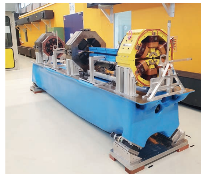
Figure 7 Demonstrator girder assembled in Building 36 on the DESY campus
