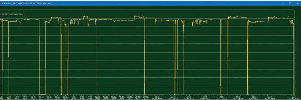
Figure 4 shows the operation history during the last quarter of 2023. Before the replacement of the cryomodules, ACC2&3 were operated at ~300 MeV, so the two renewed modules contribute to increasing the maximum electron beam energy of FLASH to 1.3 GeV. Since May 2023, user operation has visibly benefited from this increase. The beam operation of the two modules close to 250 MeV each is unique worldwide and comparable to the European XFEL.
