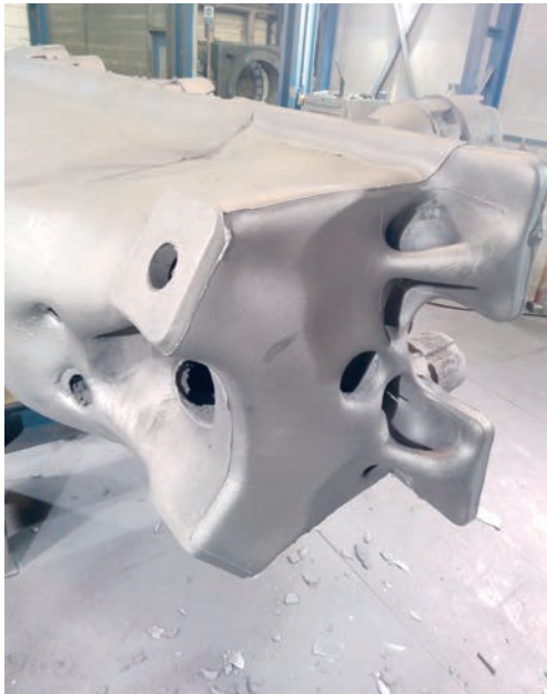
Figure 2 Left: Prototype of the novel girder design cast in metal just before Christmas 2023. Right: Final treated and painted prototype girder by COSWIG GUSS
