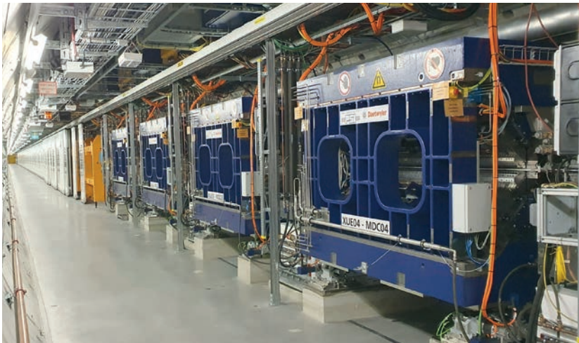
Figure 1 Left: APPLE-X undulators installed downstream of SASE3. Right: Location of the encoders on the APPLE-X undulators. Linear encoders are situated on the downstream side of the undulators, around 30 cm away from the electron beam. Rotary encoders are mounted on the motors located on the sides of the undulators at a distance of 30–40 cm from the electron beam.
