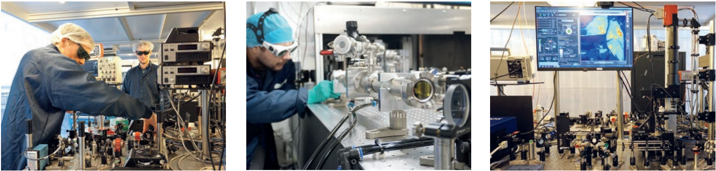
Figure 2 Left: Development of a high-power fibre laser seeding source. Centre: Installation of the newly developed beam spatial filter. Right: Multiphoton microscopy platform using an ultrashort-pulse low-noise fibre laser source.
