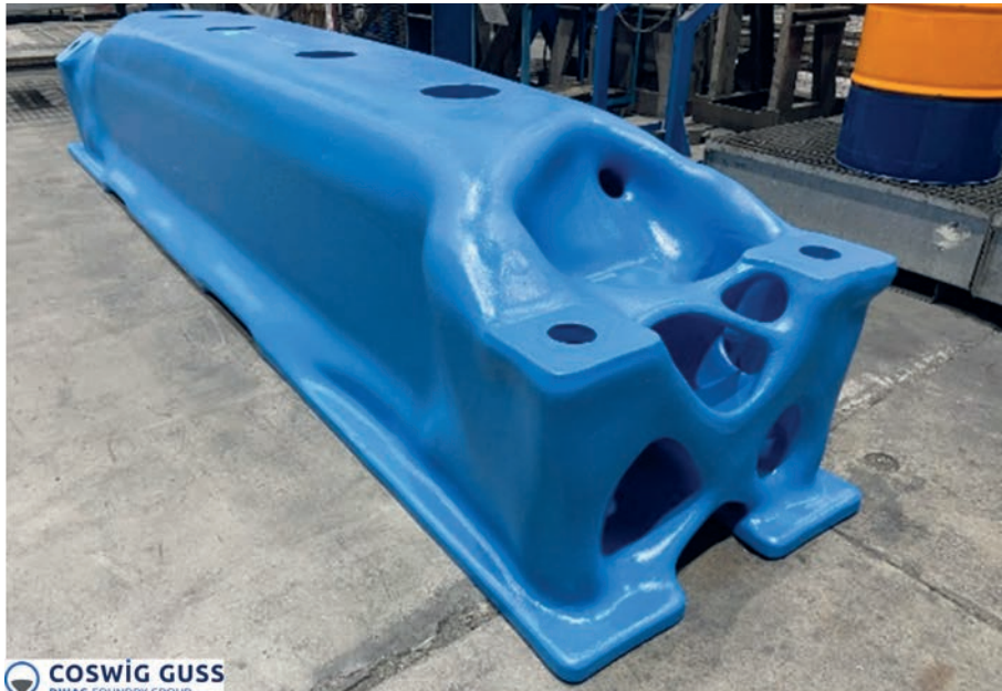
Figure 2 Left: Prototype of the novel girder design cast in metal just before Christmas 2023. Right: Final treated and painted prototype girder by COSWIG GUSS
