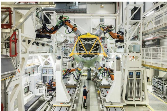
FIGURE 2: NEW AIRBUS STRUCTURE LINE A320 FOR ORBITAL JOINT [2]
