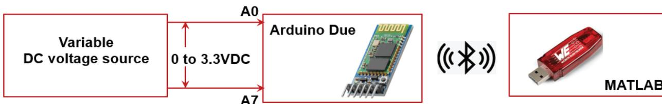
FIGURE 5: BLOCK DIAGRAM REPRESENTATION OF THE DNeD SENSOR FIRST-STEPS HARDWARE IMPLEMENTATION.
