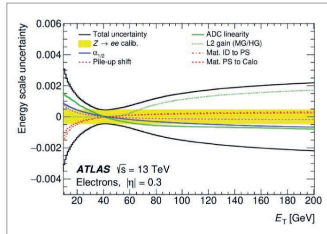
**Figure 1** Relative energy scale calibration uncertainty for electrons as a function of transverse momentum ( $E_T$ ). The total uncertainty is shown along with the main contributions. From [1].
