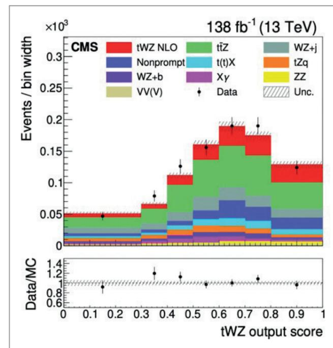
Figure 1 Output of the deep neural network classifier. The  $tWZ$  signal distribution, shown in red, is enhanced towards larger output values.
