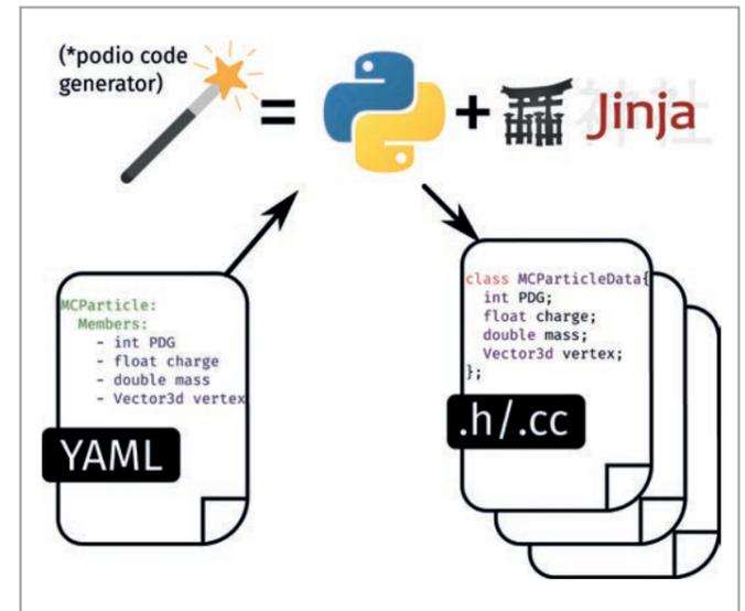
Figure 2 Flow diagram of the podio code generator, which reads a data model definition in YAML format and produces an efficient implementation in C++ as output
