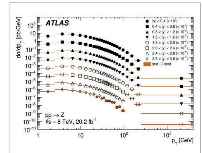
Figure 1 Measured transverse momentum of the Z boson produced in 8 TeV proton-proton collisions, in different rapidity ( $y$ ) regions. The rapidity is linked to the polar scattering angle. From [1].
