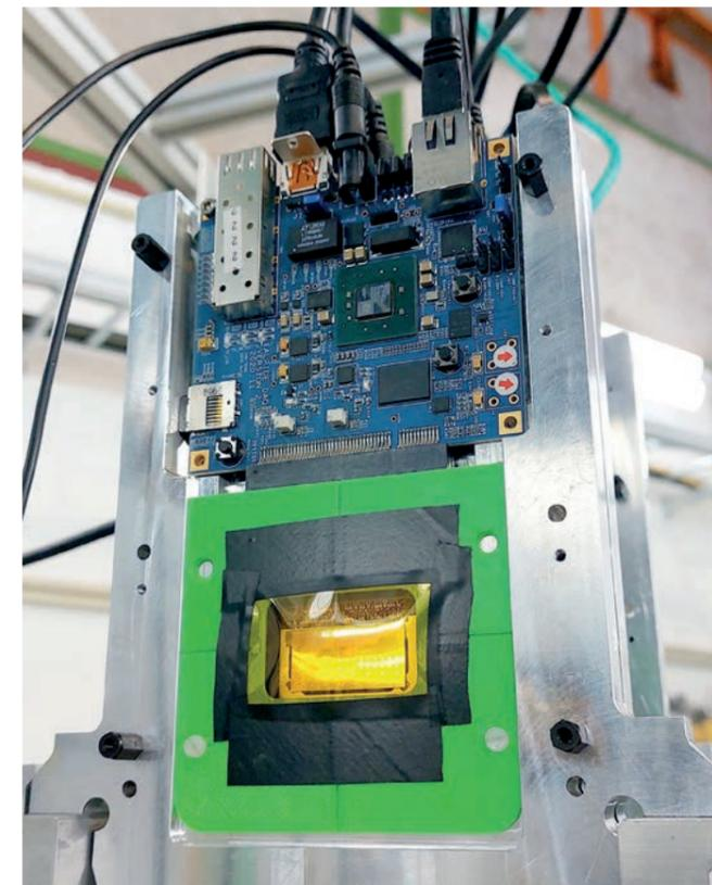
Figure 2 A layer of the new Adenium telescope prototype, with the ALPIDE pixel sensor visible behind the orange Kapton foil and the readout board on top
