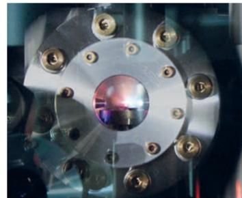
Light from the one-millimetre-long helium plasma in which the electrons were accelerated
