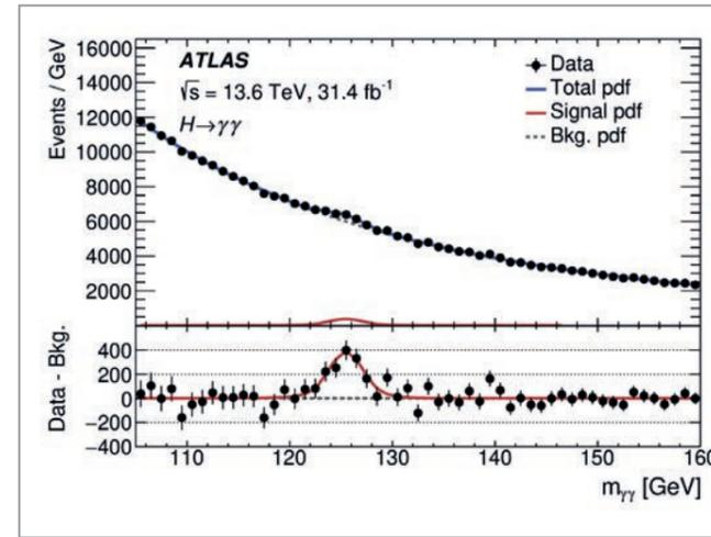
Figure 3 Di-photon invariant-mass spectrum from the  $H \rightarrow \gamma\gamma$  measurement, using data from 2022. The Higgs-boson signal peak is shown by a red line. From [4].
