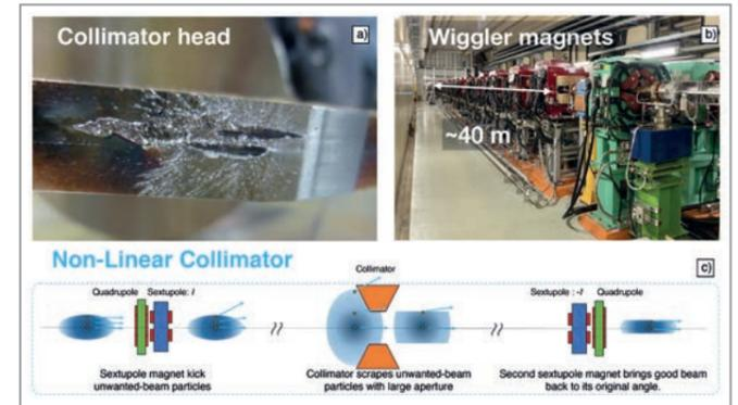
Figure 2 (a) Example of a damaged collimator head in Run 1. (b) SuperKEKB tunnel before NLC installation. (c) Schematic illustration of the NLC concept.
