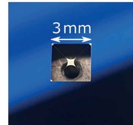
An 80 nm thick trampoline membrane made of silicon nitride is the central element of the pressure sensor.
