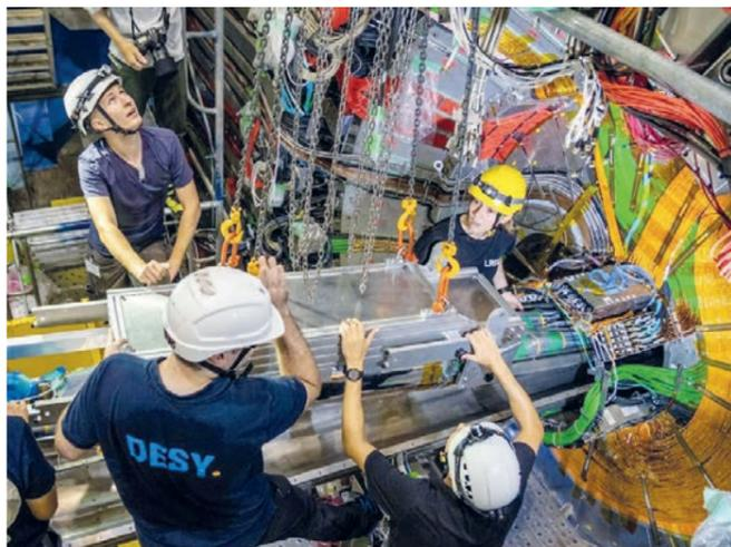
The pixel vertex detector being installed in the Belle II experiment in Japan
