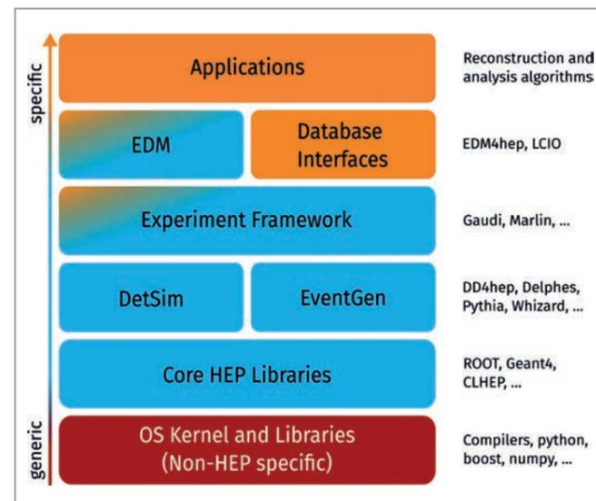
Figure 1 Schematic depiction of a typical software stack for a HEP experiment, comprising commonly available software at the base and becoming more and more experiment-specific towards the top of the stack
