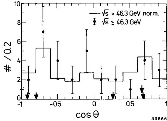
Figure 14: Muon angular distribution:  $\theta$  is the angle between the muon and the beam axis. The arrows mark the polar position of the five signal muons.
