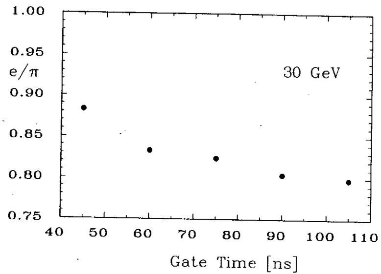
Figure 5:  $e/\pi$ -Ratio at 30 GeV as a Function of the ADC Gating Time
