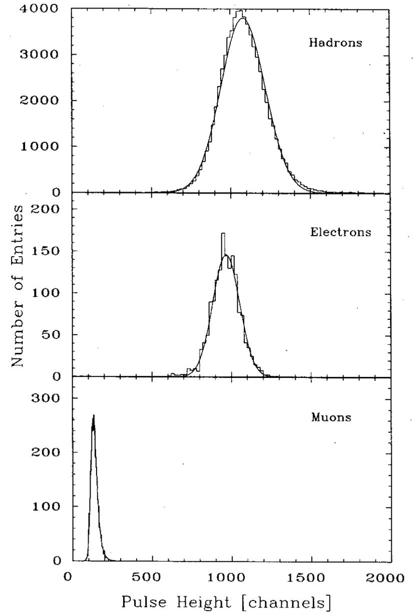
Figure 2: Hadron, Electron and Muon Response in the HAD Calorimeter at 30 GeV
