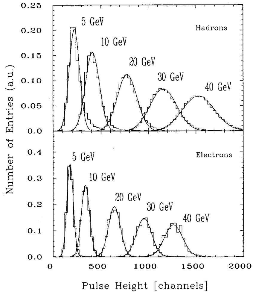
Figure 3: Hadron and Electron Response of the HAD-Calorimeter for Various Beam Energies
