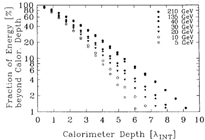
Figure 10: Cumulative Distributions of Longitudinal Energy Deposition for all Events
