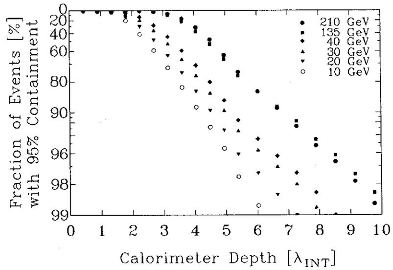
Figure 13: Fraction of Events with 95 % Containment in Calorimeter for Events with Shower Vertices in the First Module
