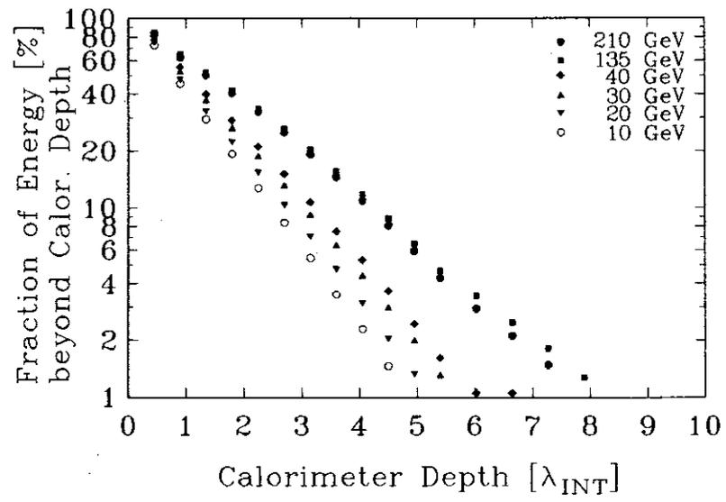
Figure 11: Cumulative Distributions of Longitudinal Energy Deposition for Events with Shower Vertices in the First Module
