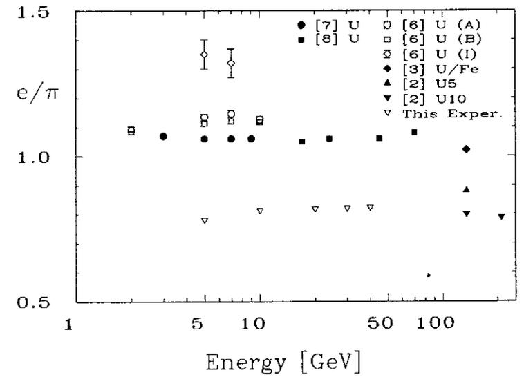
Figure 4:  $e/\pi$ -Ratio for Different Hadron Calorimeters
