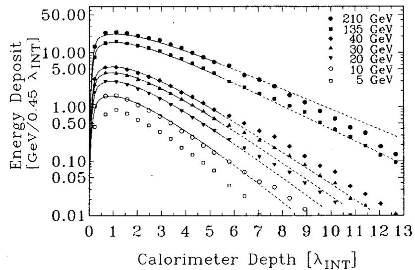
Figure 8: Longitudinal Energy Deposition for Beam Momentum of 5 to 210 GeV for all Events
