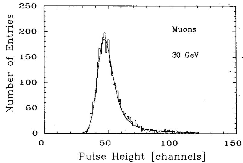
Figure 6: Muon Response at 30 GeV in the Electromagnetic Calorimeter
