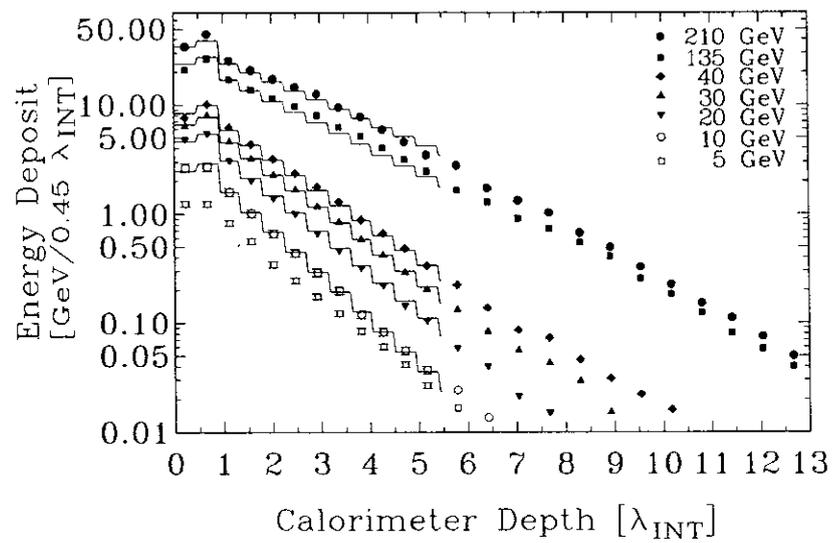
Figure 9: Longitudinal Energy Deposition for Beam Momentum of 5 to 210 GeV for Events with Shower Vertices in the First Module
