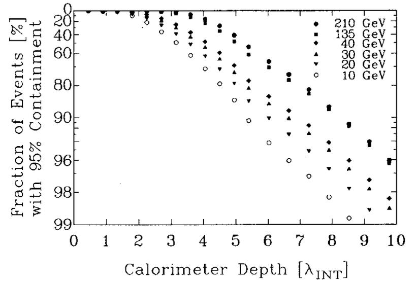
Figure 12: Fraction of Events with 95 % Containment in the Calorimeter for all Events
