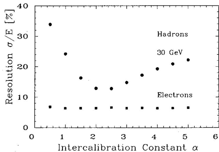
Figure 7: Energy Resolution of the Combined Electromagnetic and Hadronic Calorimeter as a Function of the Relative Calibration Constant  $\alpha$
