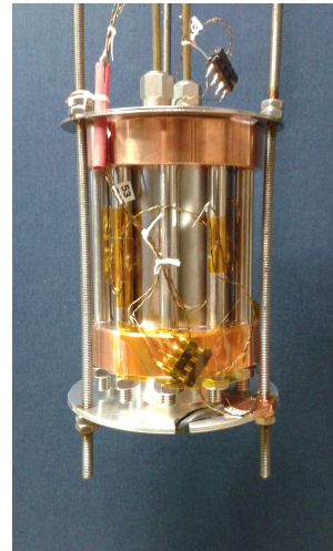
Figure 2: Nb cavity instrumented before the insertion in the LHe criostat.
