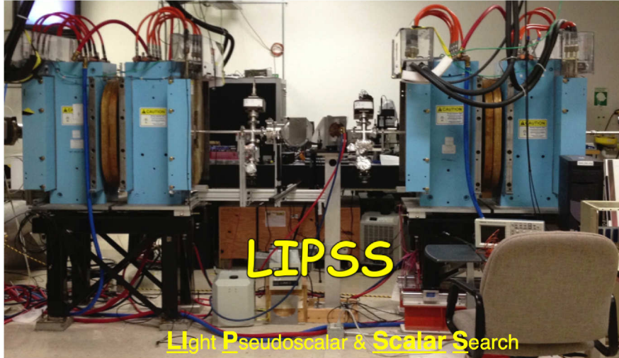
Figure 5: Image of the LIPSS experimental setup at Jefferson Lab. The dipoles are colored light blue and can be joined to form a 2 meter long, 1.7 Tesla B-Field.
