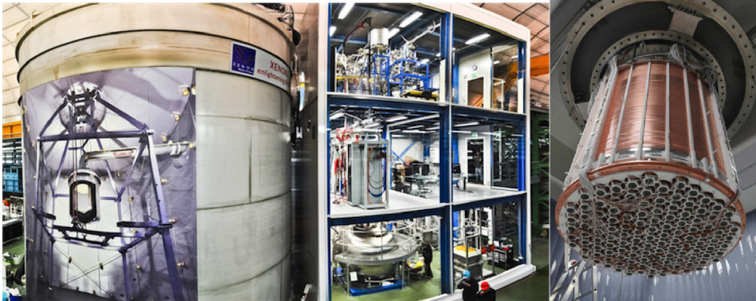
Figure 3: Left picture shows the water tank and the service building of XENON1T. Right picture shows the installed XENON1T TPC. The copper field shaping rings and the bottom PMT array are visible.
