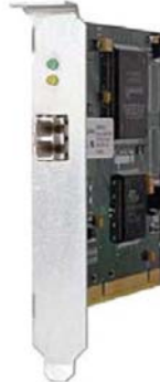
A2818 PCI CONET Controller (32 bit 33 MHz PCI-Karte)
