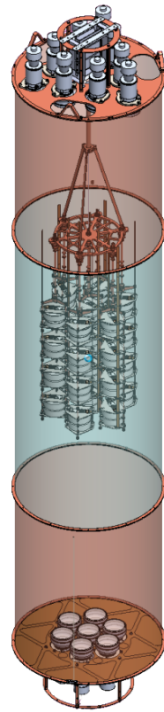
Figure 5: Schematic view of the liquid Ar veto system. Figure by courtesy of M. Heisel, MPI-K.
