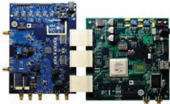
Figure 1. AD9288 and AD9289 Family Evaluation Board and HSC-ADC EVALCZ Data Capture Board
