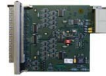
Prototype Clock and Control RTM (UCL)
