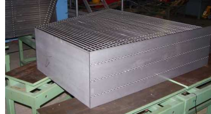
Figure 4: The vertical mechanical structure for the technical HCAL prototype.
