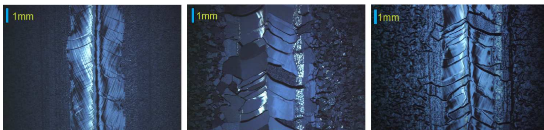
Figure 3: Equatorial welding seam of cell 1 in Z137: before EP (left), after main-EP (center) and after final-EP (right)
