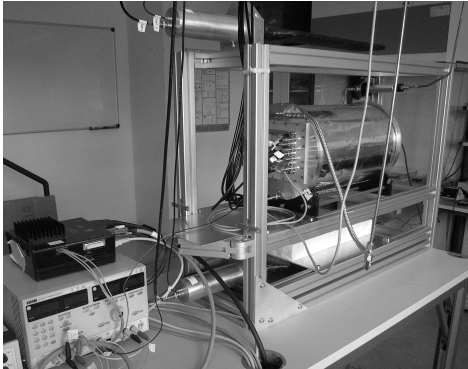
Figure 1: Detector set up in the cosmic ray test stand.
