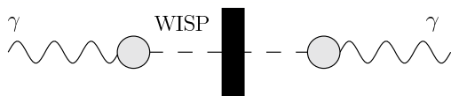
Figure 2: Sketch of a “light shining through a wall experiment”. The grey blob indicates the mixing term between photons and the “weakly interacting sub-eV particles” (WISPs).
