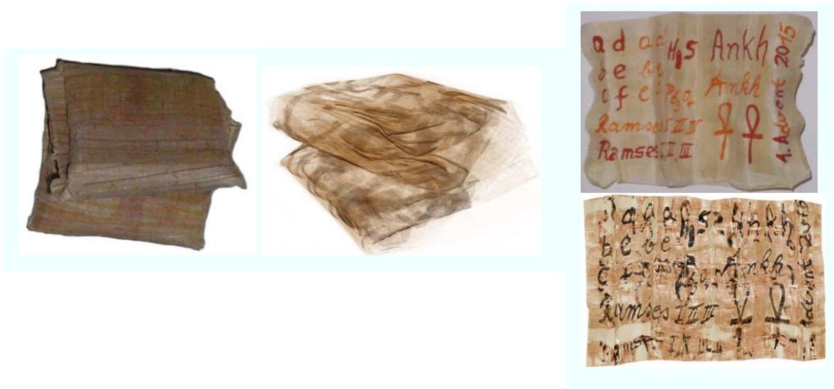
Fig 1: Photograph of the folded mockup (left), 3d-image after volume rendering using the software Amira (center), and reconstructed text (right at the bottom) compared to the original (top).
