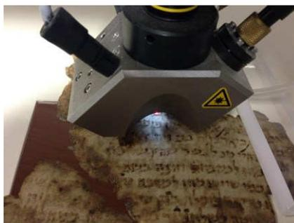
**Fig. 1:** XRF spectrometer probe above a manuscript fragment
