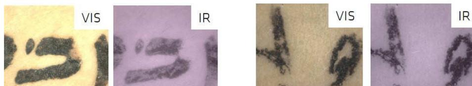
**Fig. 4:** Details of one fragment (T-S 16.124) observed with the Dino microscope (x20). On the left, when illuminated with NIR (Near-Infrared, 940 nm) light, the ink fades, indicating iron-gall ink. On the right, the image under NIR light does not change. It is carbon ink.
