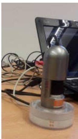
**Fig. 3:** Dino Lite digital stereomicroscope
