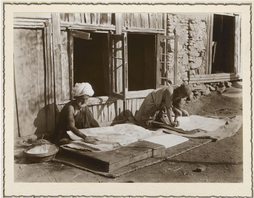
Fig 10. London, Science Museum, acquisition no. 1939-197, twenty-three photographs illustrating native paper-making in Kashmir taken by William Raitt in 1917: sizing and burnishing. © Paper Makers' Association of Great Britain.
