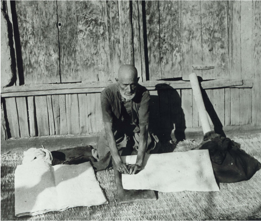
Fig. 12. Atlanta, GA, Georgia Institute of Technology, The Robert C. Williams Museum of Papermaking, paper burnishing, photograph by William Joseph ‘Dard’ Hunter (© Robert C. Williams Museum of Papermaking).
