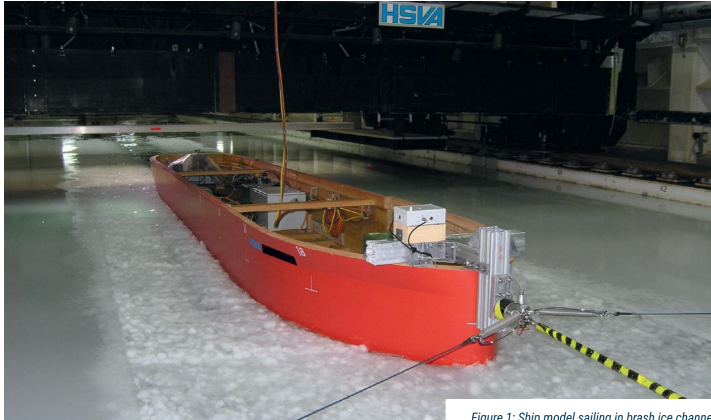
Figure 1: Ship model sailing in brash ice channel
