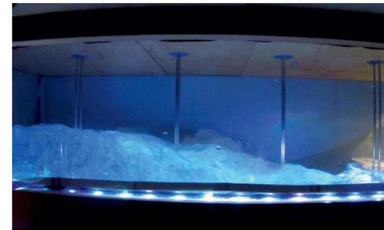
Figure 4: Dynamic water ingress in a compartment of a damaged RoPax in a transient damage case
