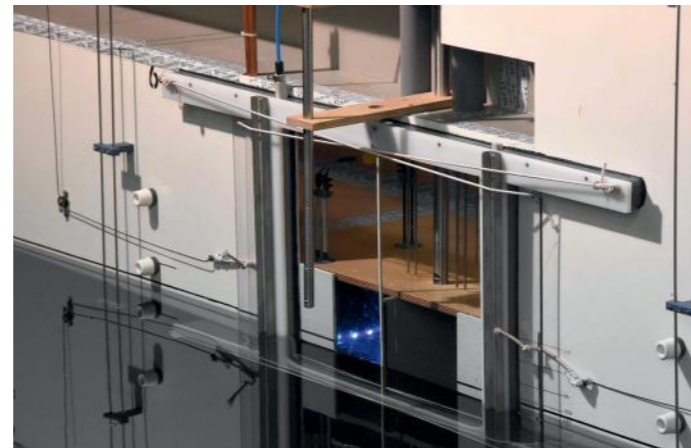
Figure 3: Controllable sliding doors for the damage opening in a transient flooding case, in which the damage opening speed cannot be ignored
