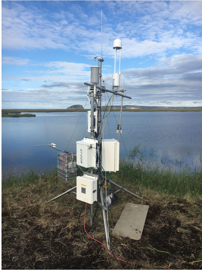
Figure 3.1: Photograph of the eddy covariance tower next to a merged polygonal pond. Since the tower was located at the shore of a large pond, it measured both tundra (westerly wind) and pond (easterly wind). The photo was taken on 11 July 2019 by the author.
