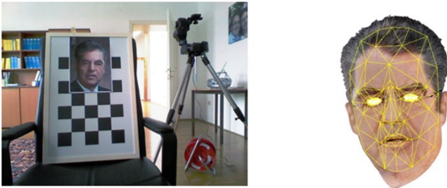
Figure 2: Face tracking with projection and high-quality face texture. Original image (left), Face texture w/ mesh (right)
