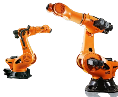
FIGURE 1: KUKA KR 1000 TITAN AS AN EXAMPLE OF INDUSTRIAL ROBOTS [5].
