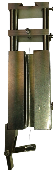
FIGURE 6. PHOTO OF A VIBRATING-WIRE SENSOR (WIRE NOT TENSIONED).
