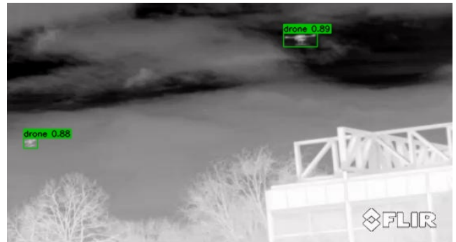
FIGURE 5. EXAMPLE RESULT FROM YOLO v5M.
