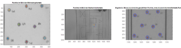
FIGURE 4 EVALUATION OF THE PRECISION OF THE REGISTRATION USING A TEST PATTERN.
