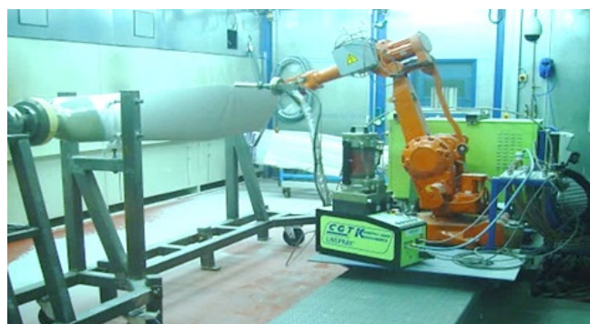
FIGURE 1. EXAMPLE OF A ROBOT-GUIDED REPAIR APPLICATION OF COLD SPRAY [3].
