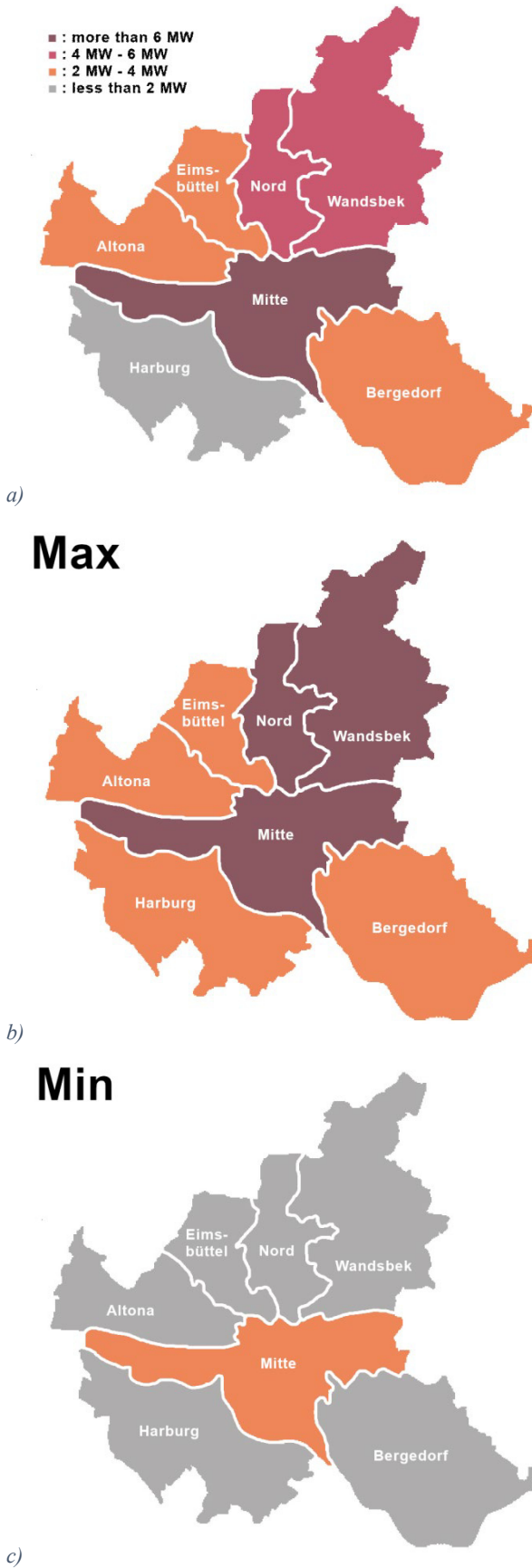
FIGURE 5: PROJECTION OF THE TOTAL PEAK DEMAND FOR THE HAMBURG BOROUGHS BY ELECTRIC TRUCK CHARGING IN 2050 (A - AVERAGE, B - MAXIMAL, C - MINIMAL SCENARIOS).
