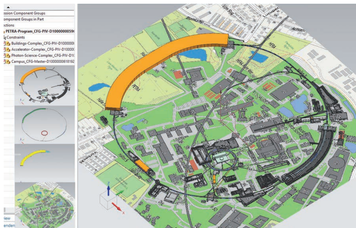
Figure 1 View of the complete integration model. Left: Building complex, accelerator complex, photon science complex and campus map shown separately.
