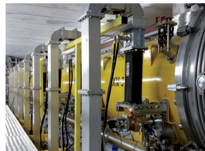
Figure 4 Cryo Module Test Bench (CMTB) facility at DESY
