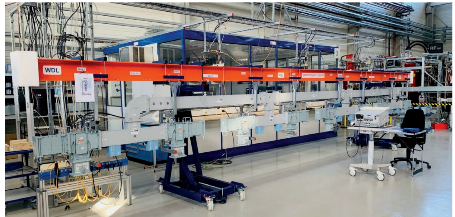
Figure 3 Complete waveguide distribution for one module on the LLRF test stand
