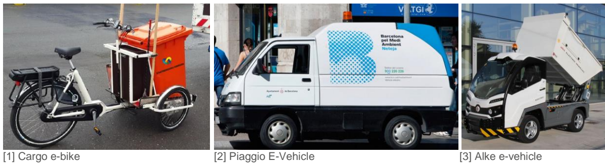
Figure 8: Examples for electric driven waste collection vehicles, (References: [1] DLR/V.Ehrler, [2] Vespa Balart, [3] Alkè)
