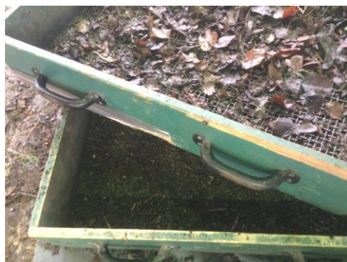
Figure 12: Bio-waste components 10-40 mm on the sieve and <10mm in the receiving container (Photo: Schermuly, 2017)
