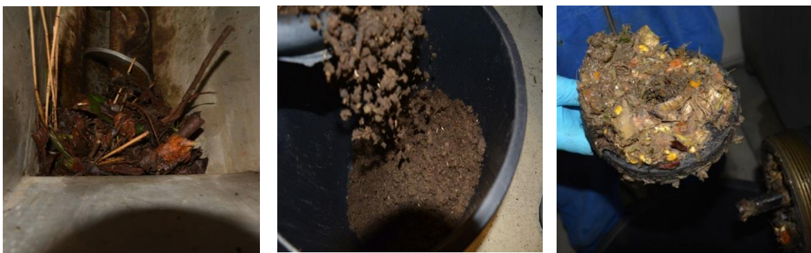
Figure 27: Obstruction found after processing garden waste (sample 1 left) in transport screw; Ground material sample 2 (green garden waste 10mm-40mm, middle); Blockage of FW (sample 3 right) in cutting section (Photos: Deegener 2017)
