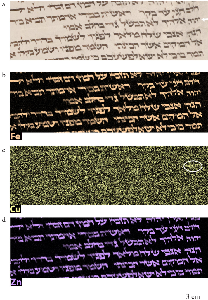
Fig. 6. Portion of sheet 19 column 1 Exodus 23,19-20; (a) image of the scanned area; (b) map of iron (Fe); (c) map of copper (Cu), with God's name marked with a white ellipse and with an arrow in the photograph; (d) map of zinc (Zn).
