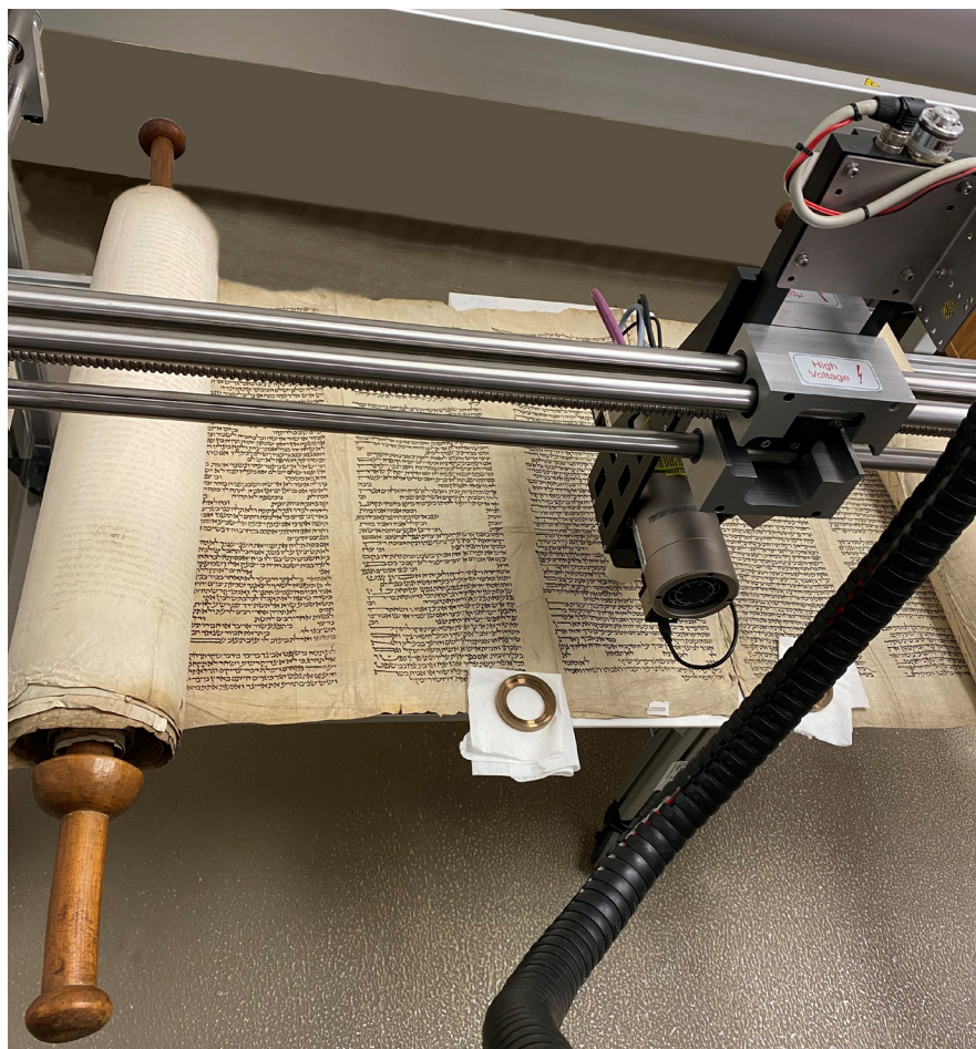
Fig. 2. The Torah scroll Erfurt 7, mounted on a custom-built aluminium stage for non-destructive measurement with a high-resolution scanning micro-XRF M6Jetstream (Bruker Nano GmbH). The scroll is partially unrolled and opened to the first column of sheet 18 and the measurement is being conducted at approximately 10 mm distance. Some additional metallic weights (at the bottom of sheet 17, column 3 and sheet 18, column 2)—separated from the surface of the scroll by acid-free paper—are being used to keep (areas that are not being measured) flat. © Staatsbibliothek zu Berlin - Preussischer Kulturbesitz, Orientabteilung, Ms. or. fol. 1216.
