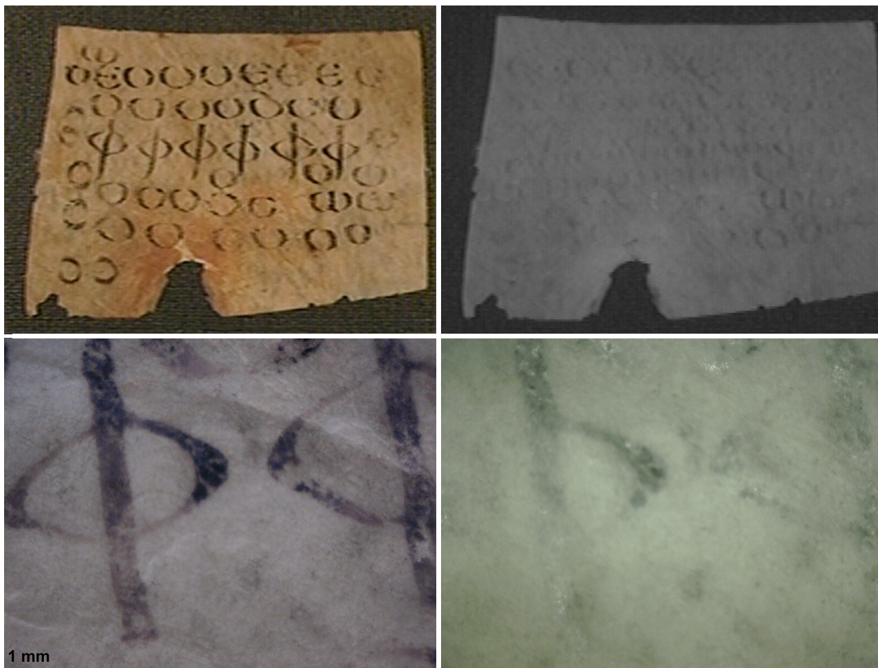
Fig. 3. Upper row: images taken with a multispectral imager in the visible region (400 – 750 nm) and near infrared region (950-1100 nm) respectively; lower row: images made with the USB microscope Dinolite in the visible region and near infrared (920-940 nm), respectively.
