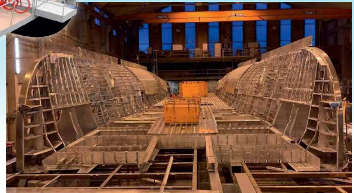
Figure 3: The Catamaran Medstraum under construction
