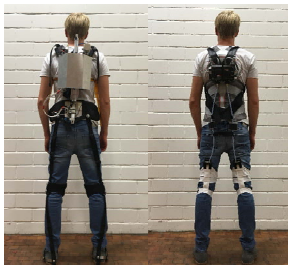
Figure 1: Overviews of two power suits developed in our lab. The left suit is pneumatically powered and is designed with a path from the shoulders to the heels. The right suit has a structure ends up at the knee and is driven by two twisted string actuators (TSAs)
