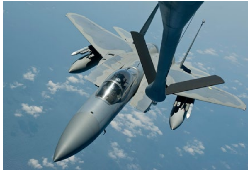
An F-15C Eagle aircraft with the 44th Fighter Squadron approaches a KC-135 Stratotanker from the 909th Air Refueling Squadron to begin an inflight refueling procedure March 21, 2016, off the coast of Japan. Copyright: U.S. Air Force photo/Senior Airman Peter Reft. Link: https://www.flickr.com/photos/usairforce/25999113016/ No changes made.
