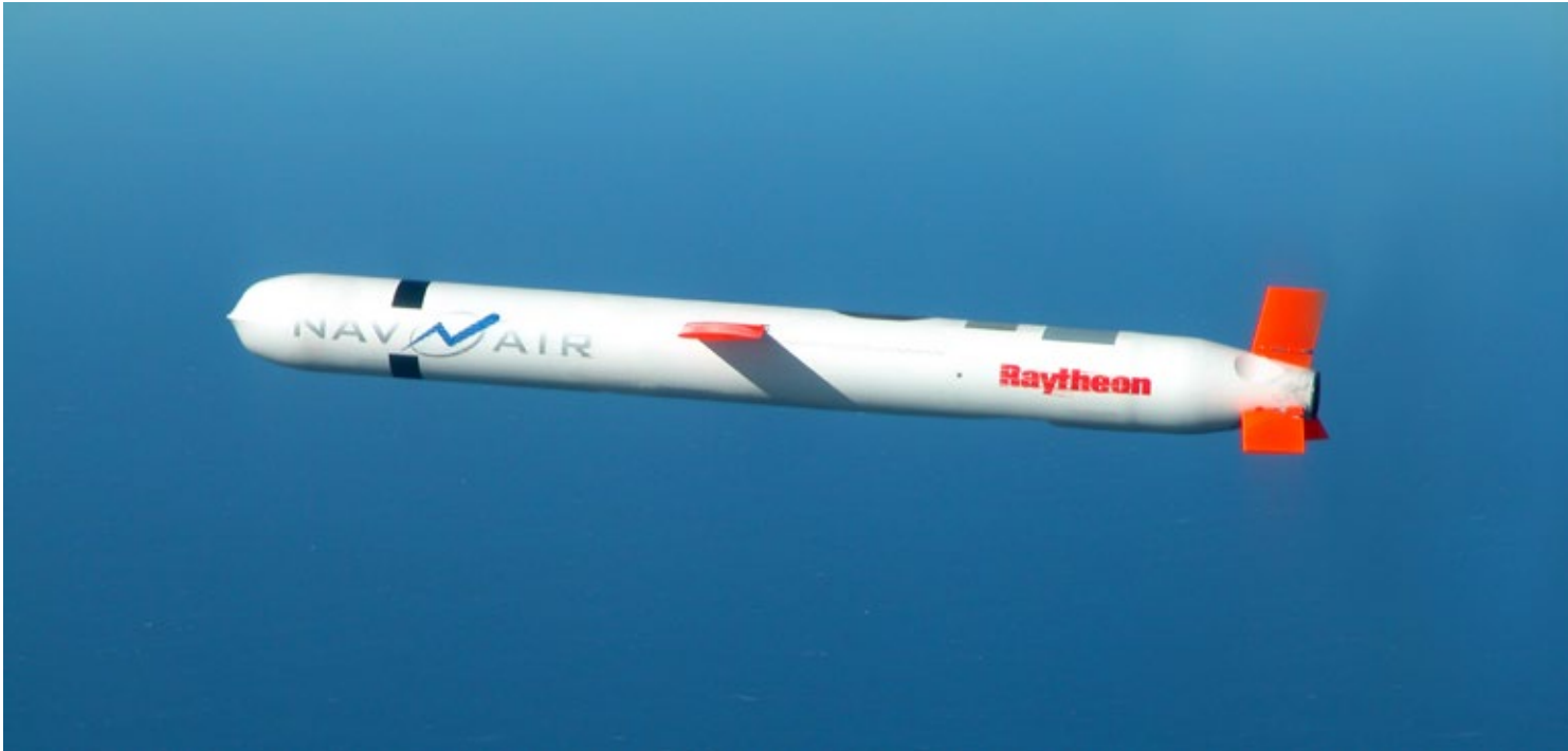
© 2002 U.S. Navy/DoD:021110-N-000X-003 China Lake, Calif. (November 10, 2002), a tactical "Tomahawk" Block IV cruise missile, conducts a controlled flight test over the Naval Air Systems Command (NAVAIR) western test range complex in southern California.
