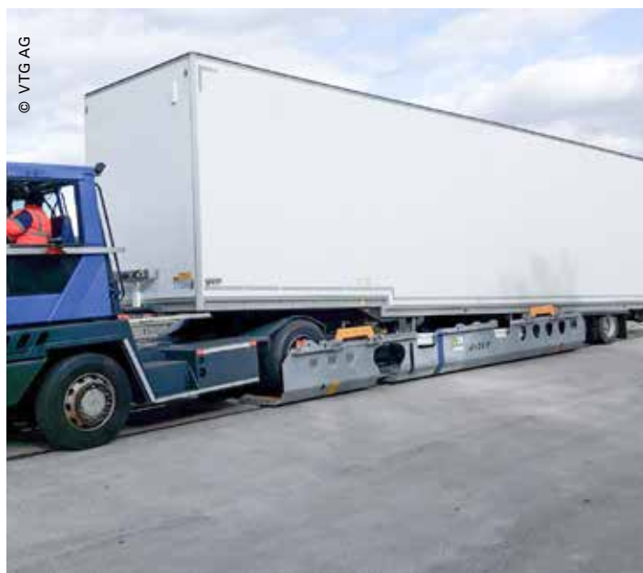
New types of semitrailers simplify the shifting of goods onto the railways.
