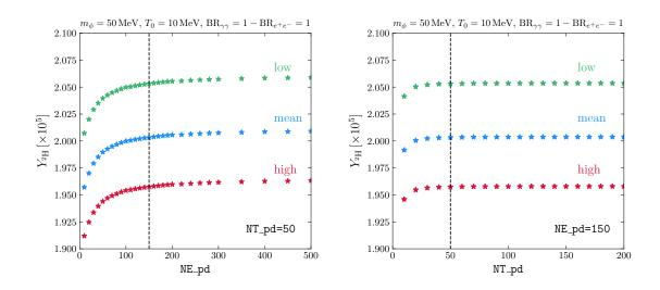
Figure 3. Convergence of the abundance of deuterium as a function of the grid points NE\_pd and NT\_pd. The dashed line indicates the default value in ACROPOLIS.
