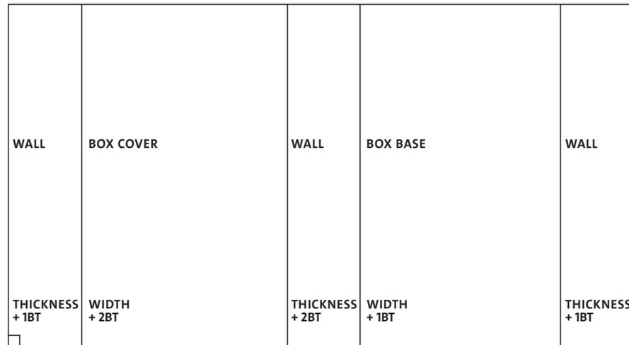
**Step 6:** Starting at the squared corner mark the horizontal dimensions as given in the drawing. Cut the board on the top using the last horizontal measurement. Using the square score the horizontal lines up to the beginning of the BOOK TRAYBASE using the pouncing wheel or a folder.
