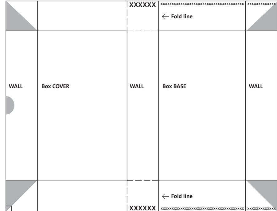
**Step 10:** Use PVA to glue the corner tabs in place. Push the inner tabs well down into the corner joints to form a sharp 90 degree angle. Allow to dry at least a couple of hours before placing the item in the box.
