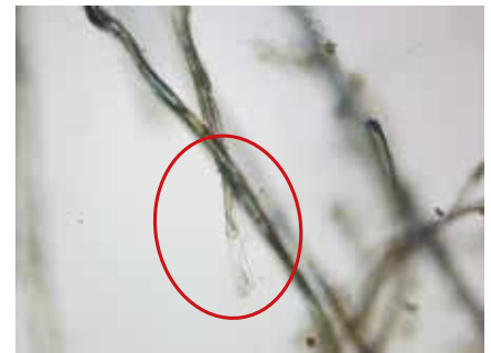
Fig. 20c: The natural fibre end enveloped by a transparent membrane, also with a natural round end, observed at 200× magnification in manuscript CMRU ARP.060 from the Chiang Mai Rajabhat University Library, Thailand.
