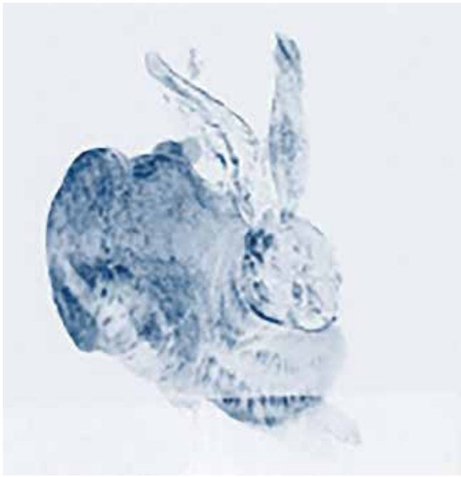
Figs. 4a, b: Element distribution images of iron (Fe) and lead (Pb). Left (a): iron; right (b): lead.
