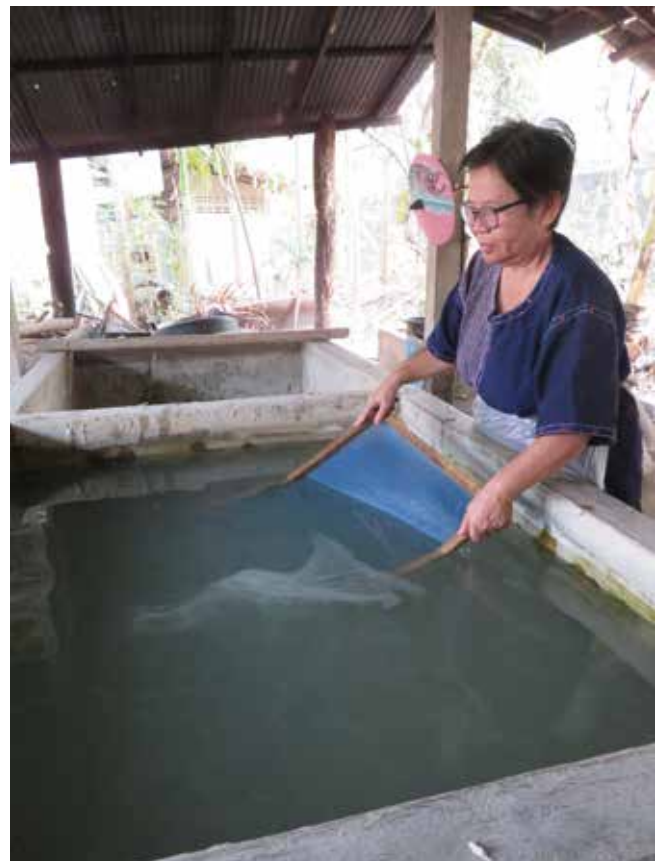
Figs 25a, b: The paper-sheet formation method using a fixed mould with a plastic screen attached to the wooden frame at Sa Paper & Umbrella Handicraft Factory, Chiang Mai. The dipping method is characterised by the paper pulp being scooped from the water tank (as opposed to the technique above, observed in Laos, where the pulp is poured directly onto the sieve in carefully measured scoops).
