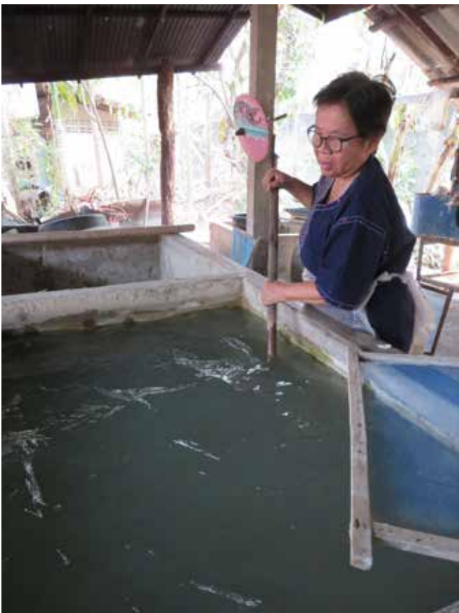
Figs 25a, b: The paper-sheet formation method using a fixed mould with a plastic screen attached to the wooden frame at Sa Paper & Umbrella Handicraft Factory, Chiang Mai. The dipping method is characterised by the paper pulp being scooped from the water tank (as opposed to the technique above, observed in Laos, where the pulp is poured directly onto the sieve in carefully measured scoops).
