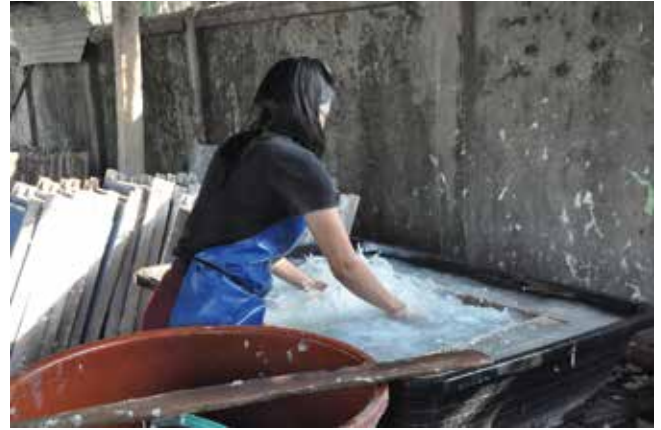
Figs 24a, b: The paper-sheet formation method using a fixed mould with a plastic screen attached to a wooden frame. Observed at Say Namkhan Company in Luang Prabang, Laos. The floating method is characterised by pouring paper pulp directly onto the sieve in carefully measured scoops (similar to a technique widely used in the Himalayas).
