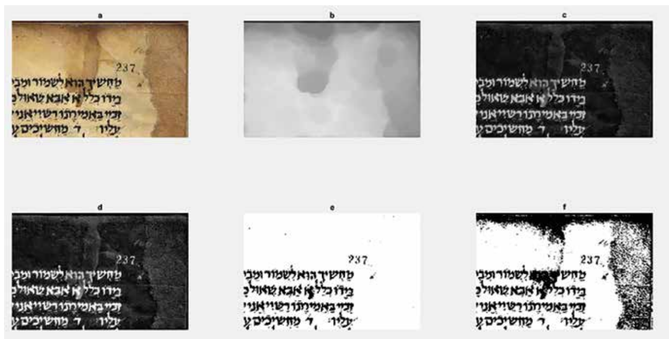
Fig. 4: Binarization process: a) input; b) closing for background calculation; c) deducing b; d) image intensity values adjustment; e) Otsu binarization and inversion of d; f) direct Otsu binarization of a for comparison.
