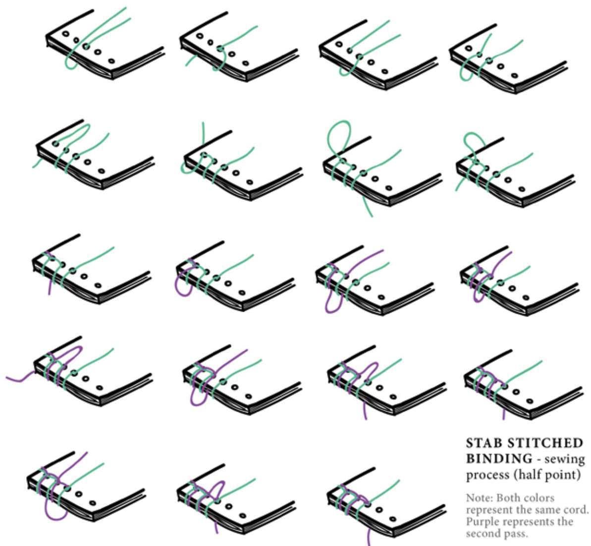
Fig. 12: The sewing process observed in stab-stitched books in Laos and northern Thailand.
