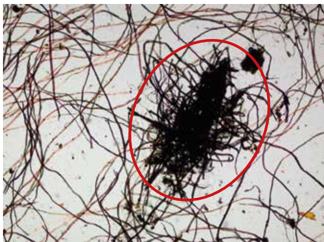
Fig. 21: A 'knot' of other fibres stained violet in paper-mulberry-based pulp. Observed at 40× magnification in the manuscript archived as CMRU Ms. 1 from the Chiang Mai Rajabhat University Library in Thailand.
