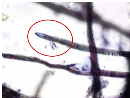
Fig. 20b: The natural blunt end of a paper-mulberry fibre after treatment with a Herzberg stain. Observed under the microscope at 400× magnification in manuscript BAD 13-2-021 from the Buddhist Archives of Luang Prabang, Laos.
