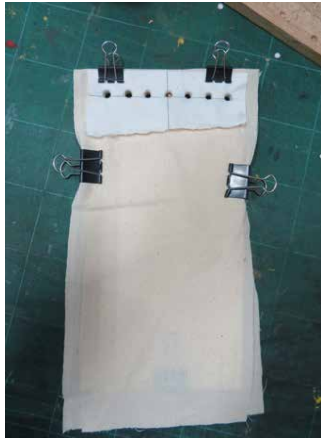
Figs 11a and b: The holes are ‘stabbed’ by using a sharp metal punch with an eye in it through which a cotton cord is then threaded. The technique is being demonstrated here by Direk Injan from the Chiang Mai Rajabhat University Library in the city of Chiang Mai, Thailand.
