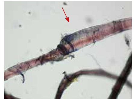
Fig. 19c: A fibre of paper mulberry enveloped by a transparent membrane after being treated with a Herzberg stain. Observed at 400× magnification in manuscript CMRU ARP.TAI 001, the Chiang Mai Rajabhat University Library, Chiang Mai, Thailand.
