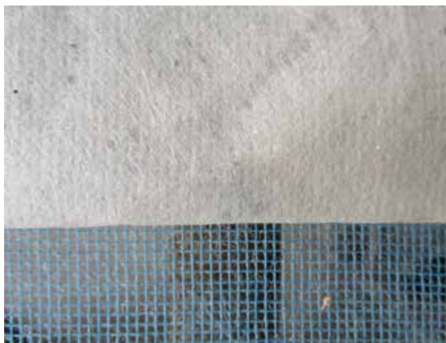
Fig. 26: The sieve imprint left on paper made using a plastic sieve attached to a wooden frame. The photograph was taken in a papermaking factory near Chiang Mai in 2020.
