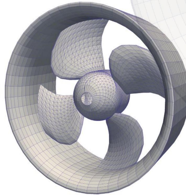
Figure 1: Panel System of Propeller and Duct
