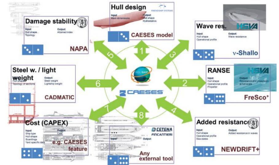
Figure 2: HOLISHIP integration concept – schema
