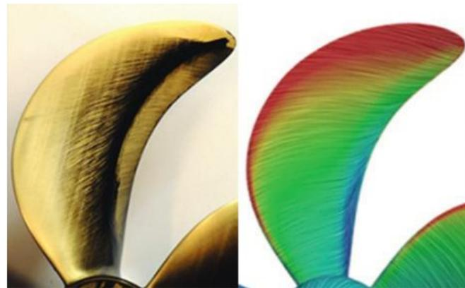
Figure 3: Flow visualisation by EFD/CFD
