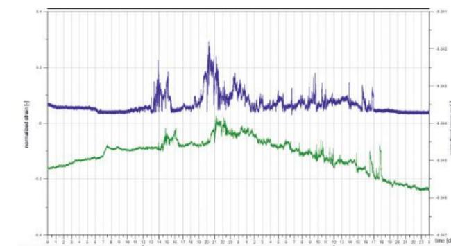
Figure 4: Measurement of the shear strain at Frame 2, Position 1 plotted together with the ice pressure at Panel 2, Zone 1 over the 2nd and 3rd of December 2019 [4]
