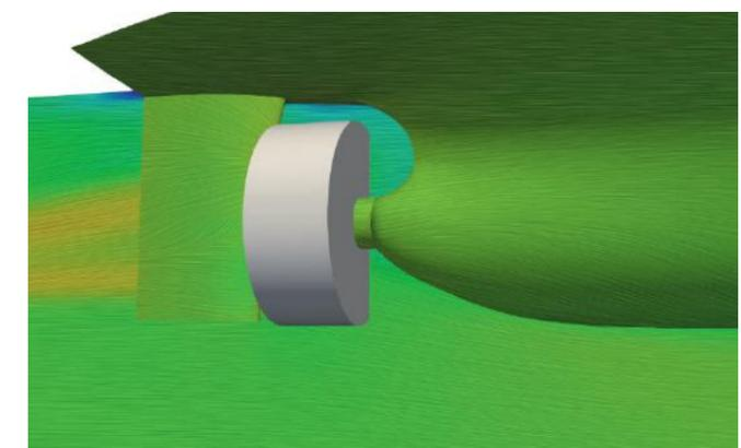
Figure 1: View onto the stern of NAWIGATOR XXI and the cylinder (grey) containing the actuator disk
