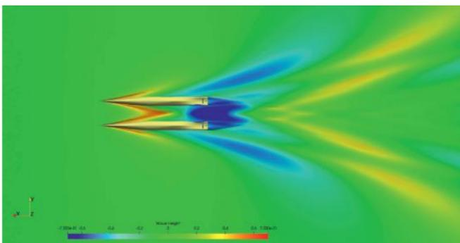
Figure 3 (left): Free surface deformation at 23 knots
