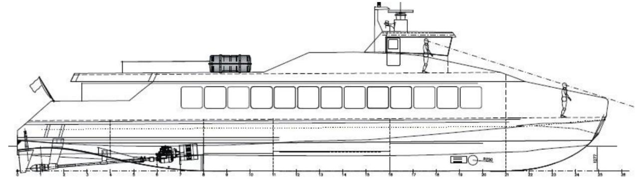
Figure 1: Preliminary general arrangement of the Stavanger Demonstrator
