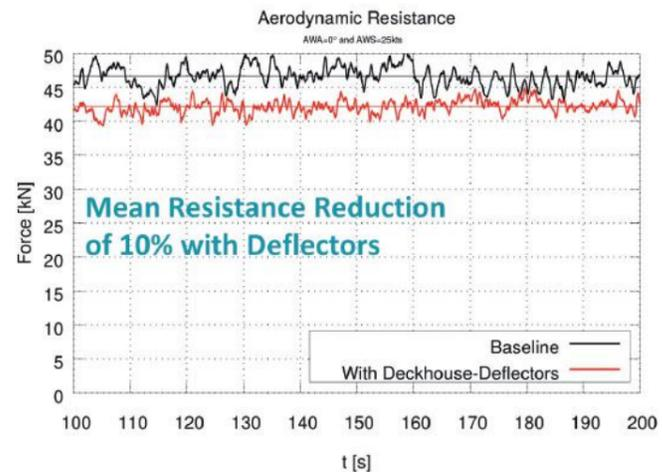
Figure 4: Total aerodynamic resistance for the 1000 TEU container vessel with stowage
