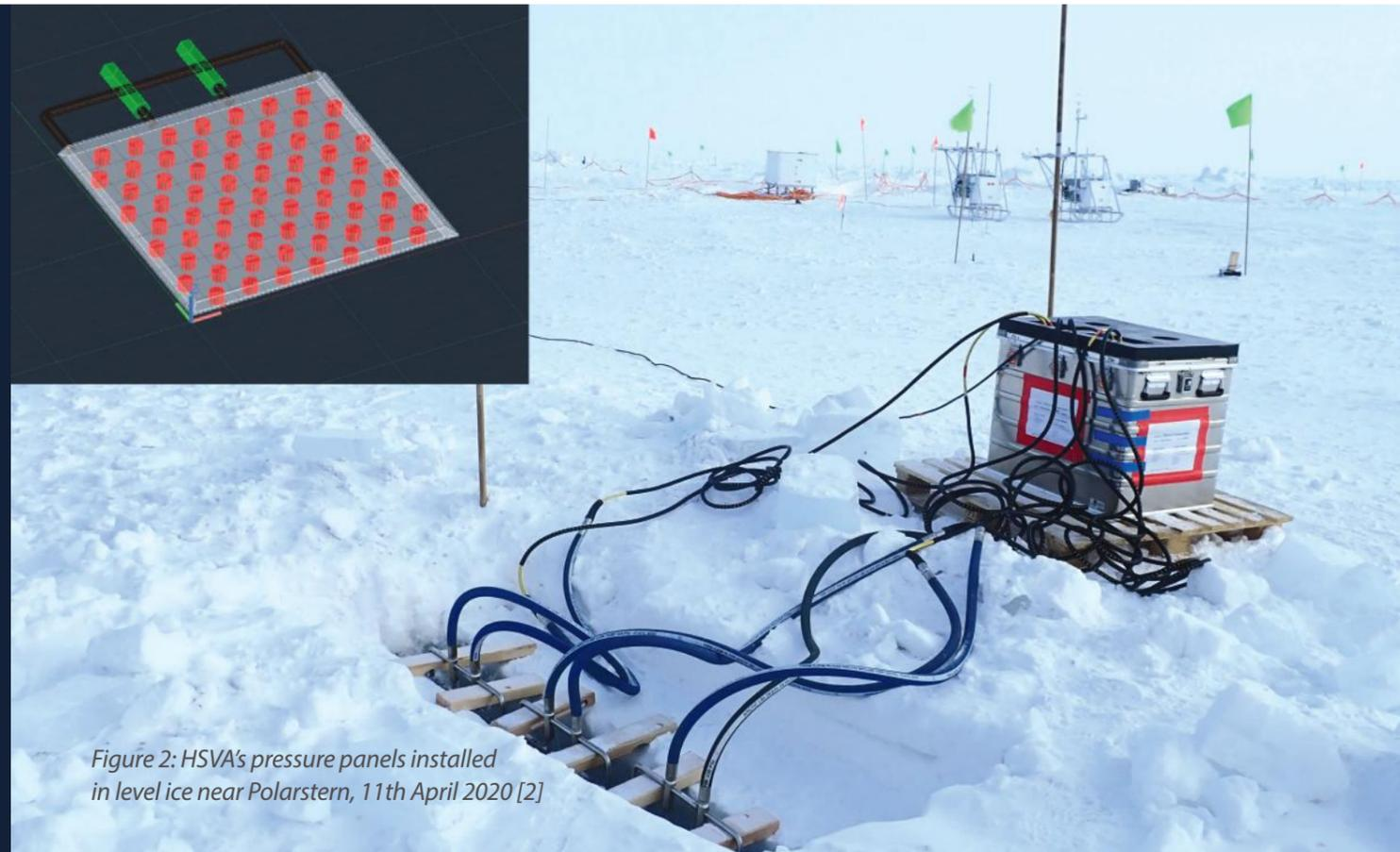
Figure 2: HSVA's pressure panels installed in level ice near Polarstern, 11th April 2020 [2]
