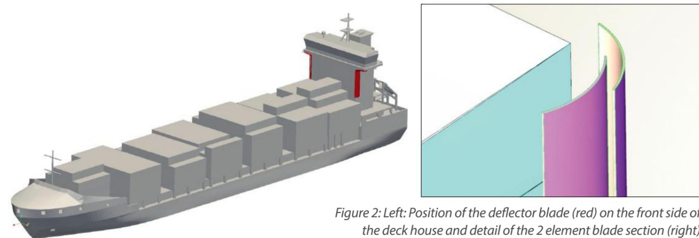
Figure 2: Left: Position of the deflector blade (red) on the front side of the deck house and detail of the 2 element blade section (right)
