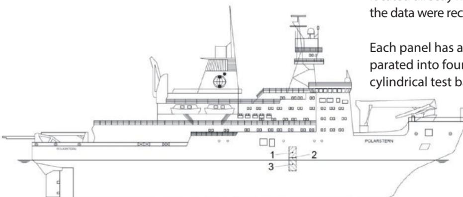
Figure 3: Strain measuring locations on Polarstern, 1 Void Space 100, 2 F-Deck 2, 3 Void Space 92 [3]
