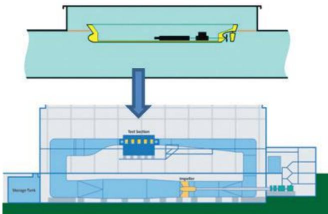
Figure 2: HYKAT with installed ship model
