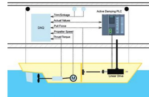
Figure 1: Principle design of the active damping system
