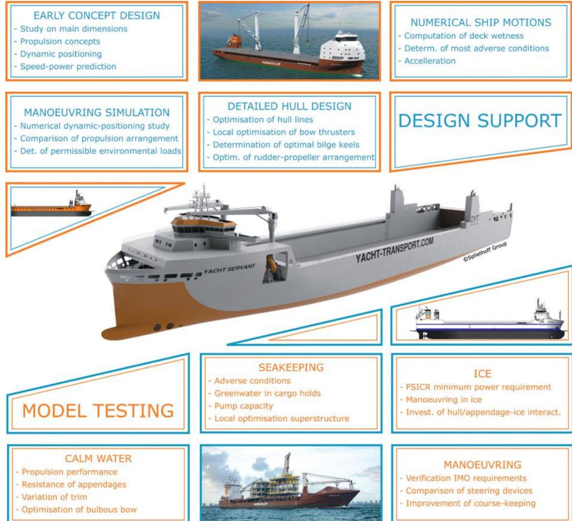
Selected services in the context of the design phase and the model test phase are shown in the enclosed graphic.
