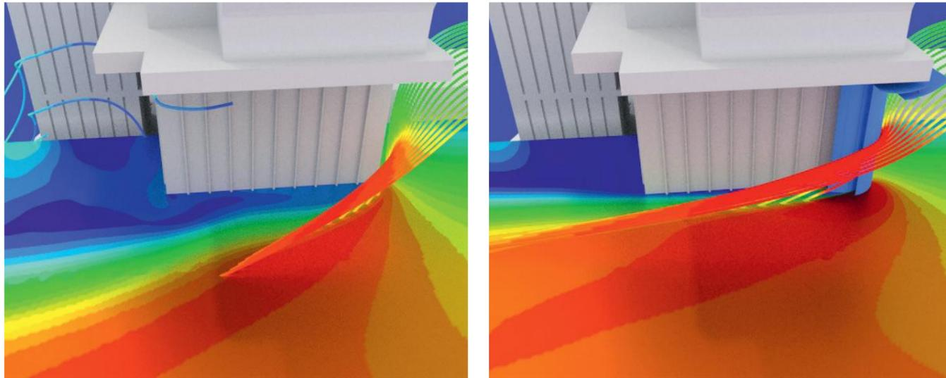
Figure 3: Improvement of corner flow on the front edge of the deck house using deflector blades
