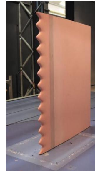
Figure 2: Wing with contoured leading edge to increase the maximum lift angle
