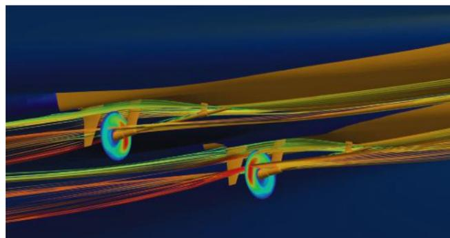
Figure 4 (right): Streamlines through propeller disc and propeller body force distribution at 23 knots
