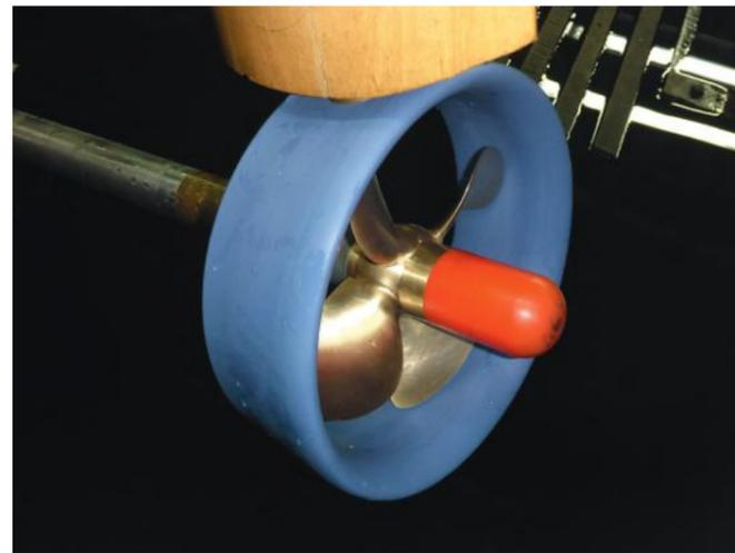
Figure 3: Model test of propeller and duct
