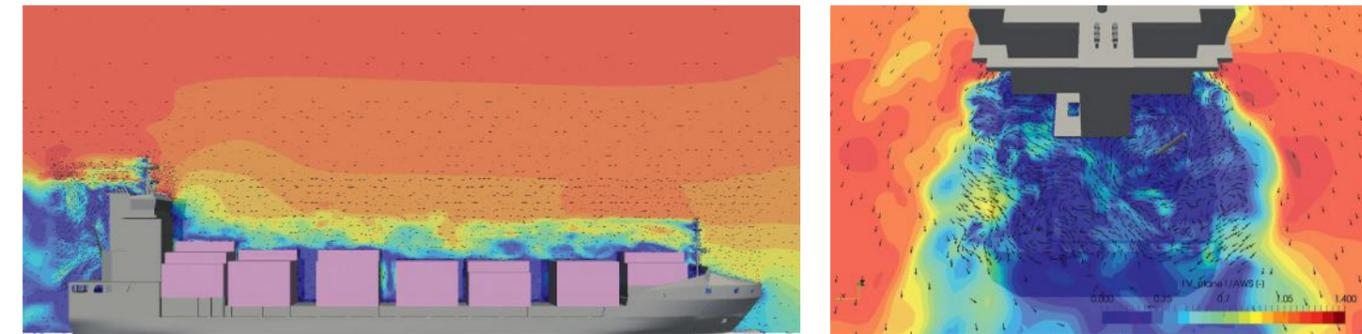
Figure 1: Instantaneous turbulent flow field in a vertical plane at center line (vxz left) and in a horizontal plane 20 m above baseline through the deck house (vxy right), obtained from a DES-simulation
