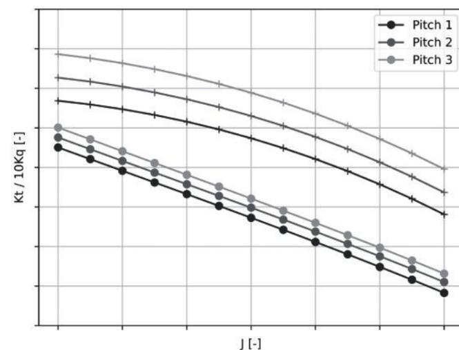
Figure 2: Computed open water characteristics with different pitch settings
