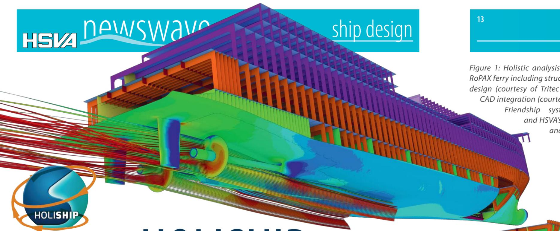
Figure 1: Holistic analysis of a RoPAX ferry including structural design (courtesy of Tritec Ltd), CAD integration (courtesy of Friendship systems) and HSVA's CFD analysis
