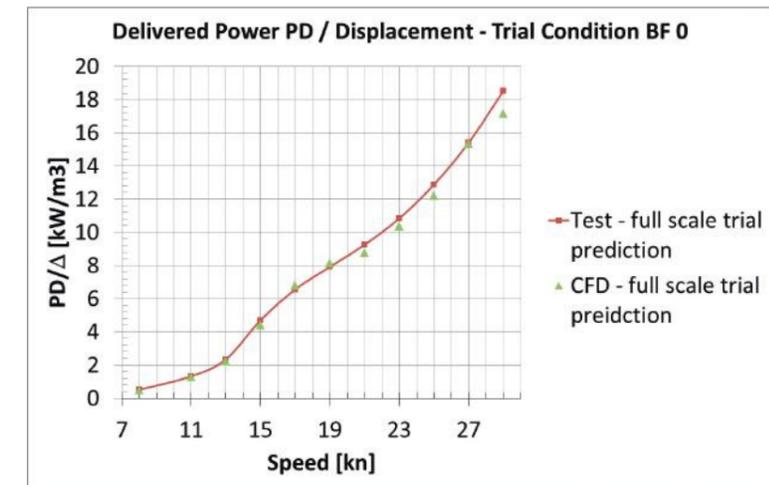
numerical CFD predictions. A comparative speed-power diagram, with the delivered power scaled with the catamaran's displacement, is shown in Fig. 6.
