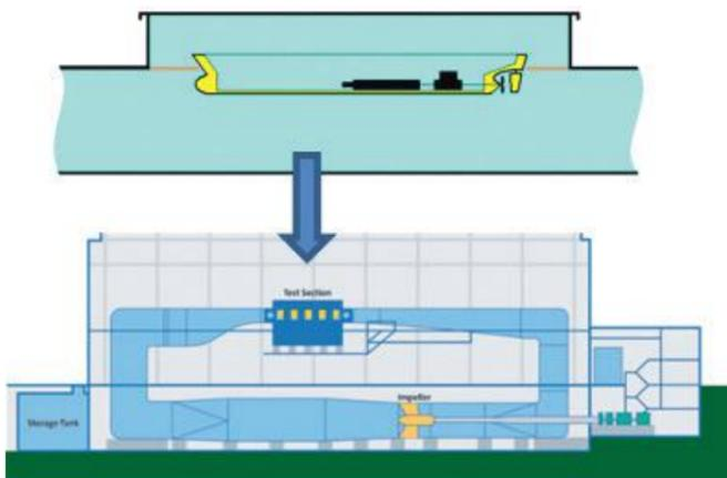
Figure 2: HYKAT with installed ship model
