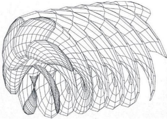
Figure 2: Lattice representation of the propeller and its slip stream
