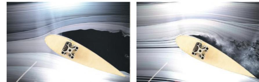
Figure 3: Delay of flow separation by active flow control
