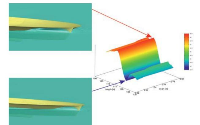
Figure 3: Parametric hullform optimisation for a double ended ferry
