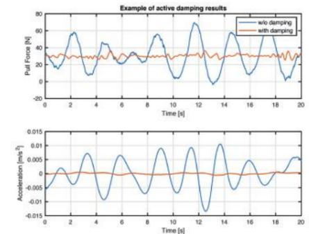
Figure 2: Effect of active damping on the signal characteristics
