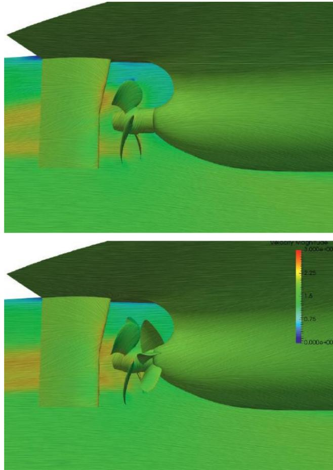
Figures 3, 4: View of the stern of NAWIGATOR XXI w/o and with PSS and the resolved propeller via sliding grid technique
