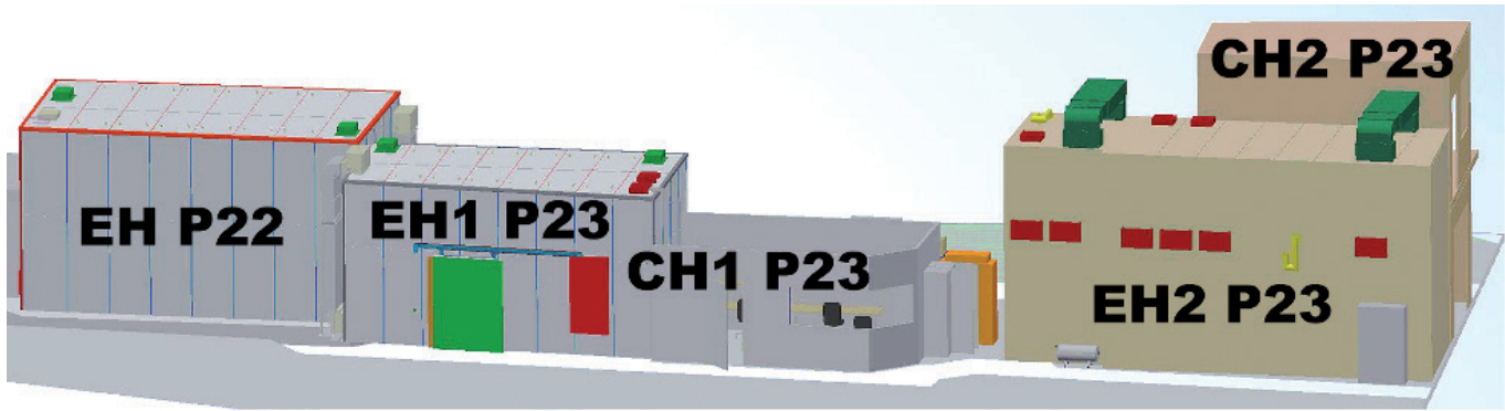
Figure 4 Completed design of the new hutches EH2 and CH2 to add hierarchical imaging capabilities to the PETRA III beamline P23. (Drawing: Design by KIT, Karlsruhe, Germany)
