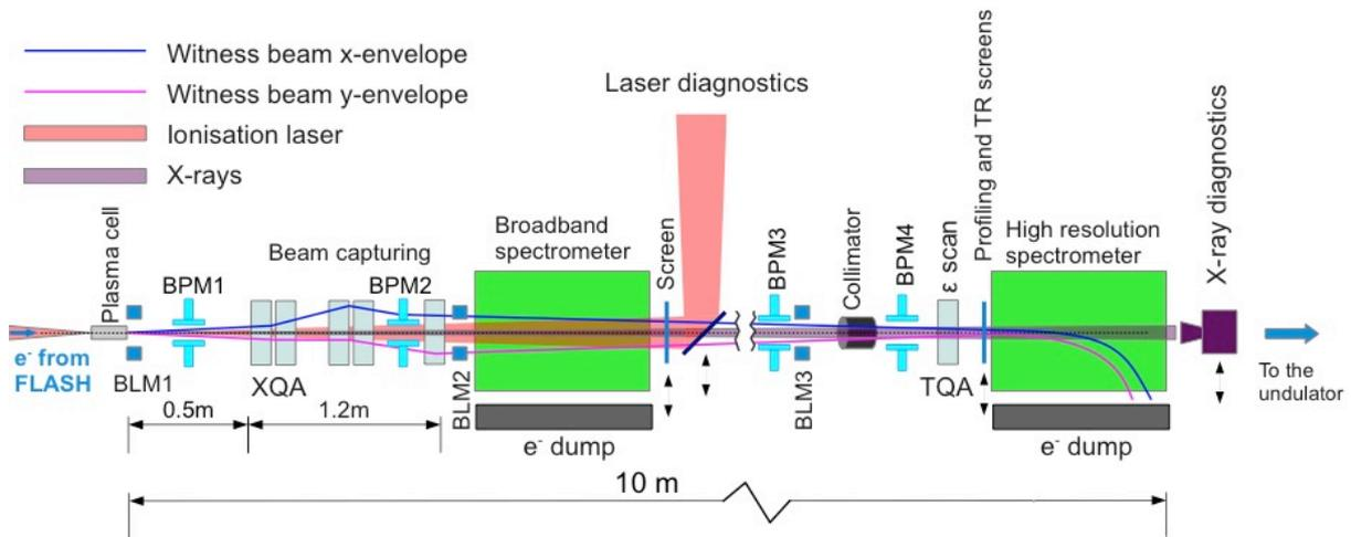
Figure 5 – Post-plasma beamline layout: BPM stands for beam position monitors, BLM is the beam loss monitor while XQA/TQA denote electromagnetic quadrupoles.
