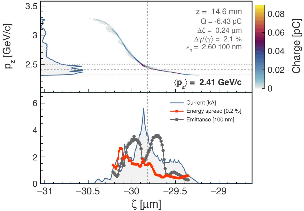
Figure 8 – Witness electron bunch injected in the plasma wake by means of wakefield-induced ionisation injection, after  $\sim 14$  mm of acceleration in plasma. (a) Longitudinal phase-space of the beam together with its projection on the  $p_z$  axis. (b) Current profile of the beam (solid line), sliced energy spread (squares), and sliced normalized emittance in the horizontal plane (dots). Units are as indicated in the panels.
