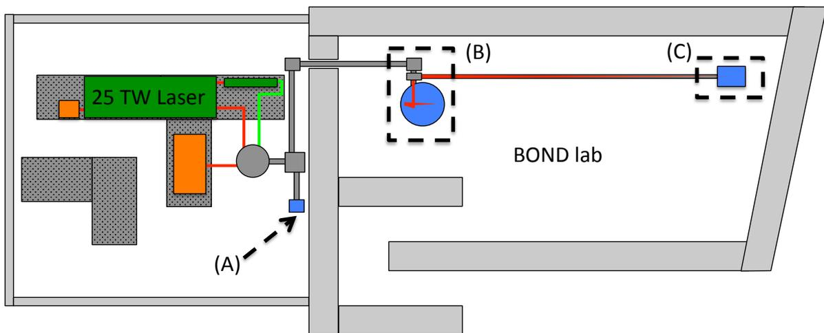
*Figure 6* – Laser and preparation laboratories for FLASHForward, consisting of laser lab, and BOND lab with 1 metre thickness concrete wall for shielding. (A) Laser output to FLASHForward beamline, (B) BOND experimental chamber (C) Ionisation test chamber.
