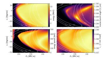
FIG. 4. Final bunch energy, inverse bunch length, energy spread, and normalized transverse emittance for the matched case,  $(B_1, z_s)$ =(0.179 T, 10.5 cm). In each case we overlay the final bunch charge as white contour levels for 0.3, 0.6 and 0.9 charge transmission. While all final energies are approximately equal (~11 MeV), the structure allows for the production of widely-tunable electron beams.
