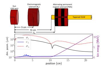
FIG. 1. Diagram of the accelerator concept (top) and corresponding evolution of the bunch's transverse emittance ( $\varepsilon_r$ ), rms transverse beam size ( $\sigma_r$ ), longitudinal bunch length ( $\sigma_z$ ) (all left axis) and the kinetic energy (right axis) along the accelerator beamline (bottom). The example corresponds to an operating point ( $\phi$ ,  $E_0$ )=(79.3 deg, 106.875 MV/m); see text for details.
