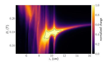
FIG. 3. Charge fractional transmission through the structure as a function  $B_1$  and  $z_s$  for injection parameters ( $\mathcal{E}_i$ ,  $E_z$ )=(205 keV, 105.8 MV/m) corresponding to a maximum bunch compression point from Fig. 2(c). A black dashed line encompasses 100% transmission.
