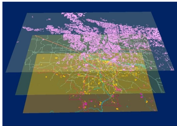
Another view of the same Portland, Oregon GIS data: residential parcels (top), transportation network (middle), and commercial and industrial parcels (bottom). A total of 371,300 land parcels are rendered in 3D in this figure, while the digital transport network has 130,141 arcs and 104,048 nodes.
