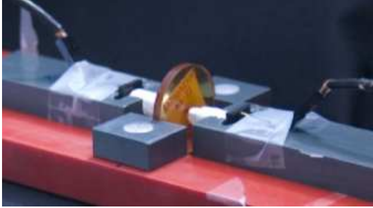
Fig. 1. Setup for the energy and time resolution measurements of LSO crystals. The scintillators (white) are directly read out by the MPPC and aligned with a ^{22}\text{Na} source positioned in the middle. The setup allows a reproducibility of the measurements of 3% for the 3 \times 3 \text{ mm}^2 detectors and 10% for the 1 \times 1 \text{ mm}^2 ones.
