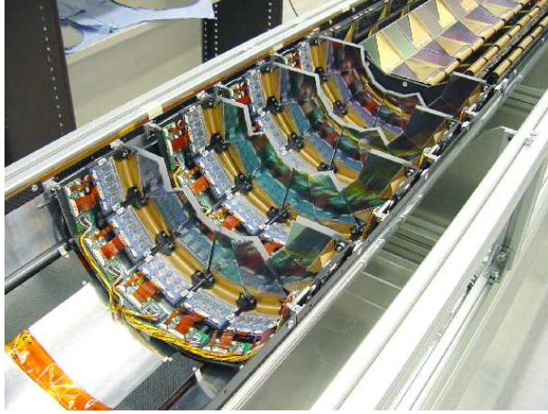
Fig. 17. Half wheels installed in the overall support structure
