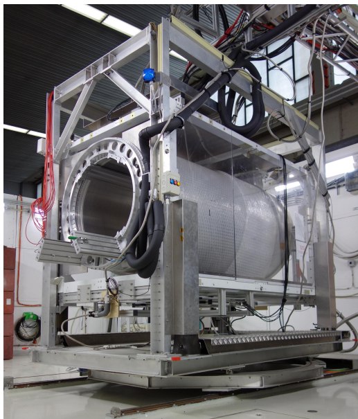
Figure 20: (Colour online) TB24/1 test beam area at DESY: movable lifting stage with the PCMAG 1 T solenoid.
