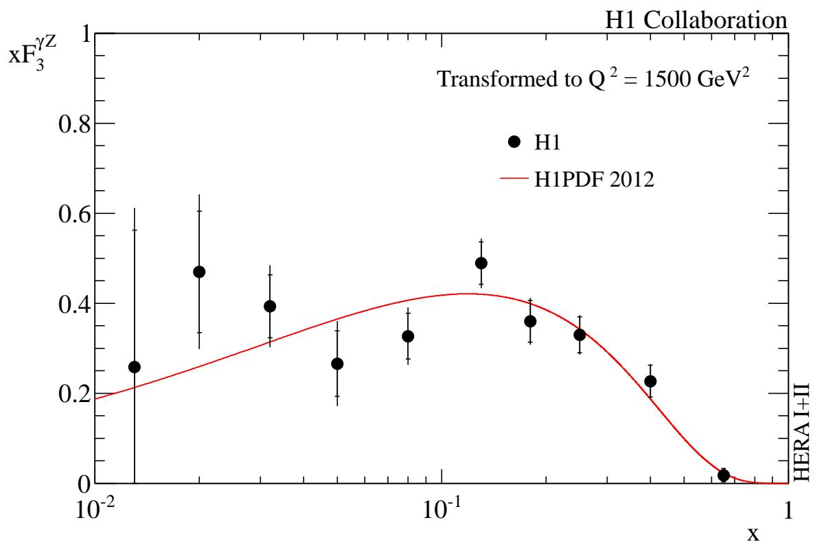
Figure 28: Structure function  $x F_3^{\gamma Z}$  transformed to  $Q^2 = 1500 \text{ GeV}^2$  for data (solid points) and the expectation from H1PDF 2012 (solid curve). The inner error bars represent the statistical uncertainties and the full error bar corresponds to the total measurement uncertainty.
