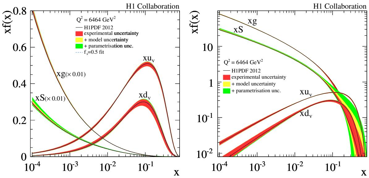
Figure 19: Parton distribution functions of H1PDF 2012 at the evolved scale of  $M_W^2$ . The gluon and sea distributions in the linear scale plot (left) are scaled by a factor 0.01. The PDFs with  $f_s = 0.5$  are also shown. The uncertainties include the experimental uncertainties (inner), the model uncertainties (middle) and the parametrisation variation (outer). All uncertainties are added in quadrature.
