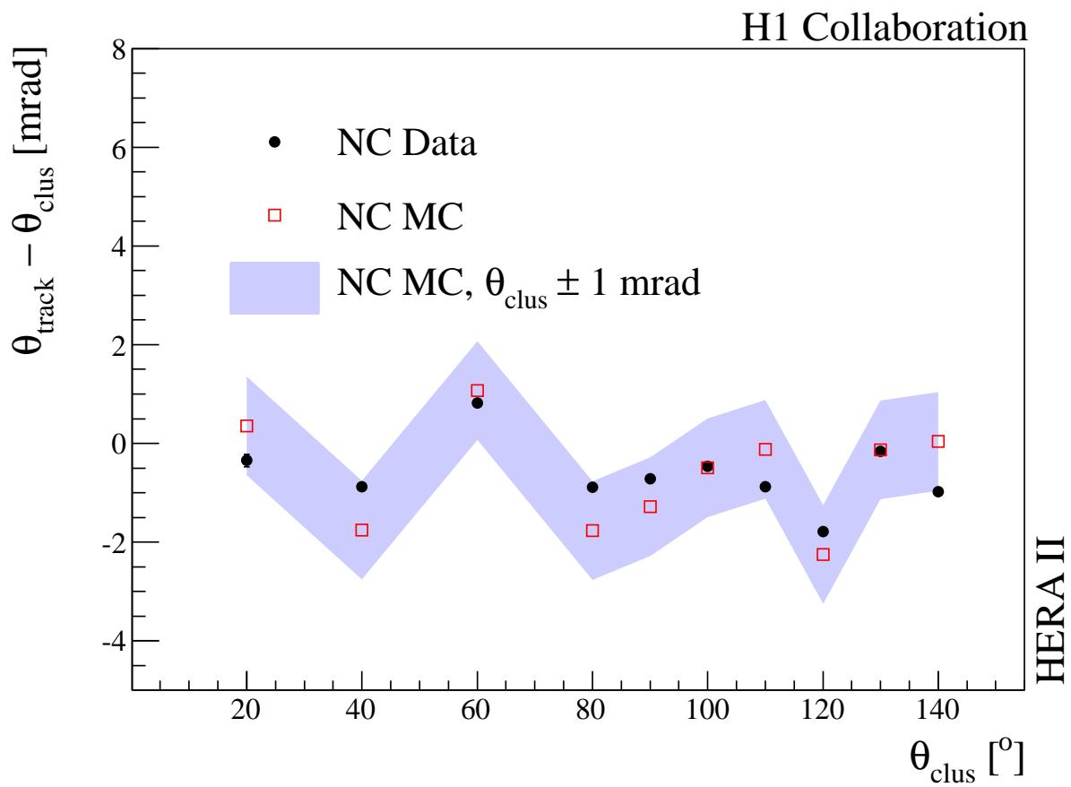
Figure 1: The mean value of  $\Delta\theta = \theta_{\text{track}} - \theta_{\text{clus}}$  as a function of the polar angle of the cluster  $\theta_{\text{clus}}$  after alignment for data (solid points) covering the complete HERA II data set and simulation (open squares). The shaded band corresponds to a  $\pm 1 \text{ mrad}$  uncertainty.
