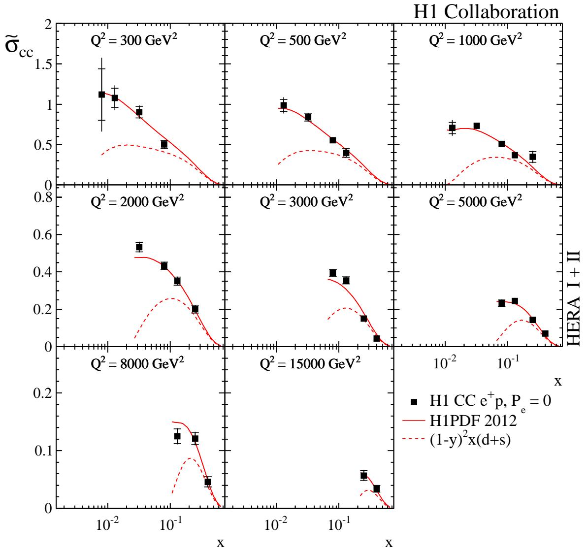
Figure 16: Combined HERA I+II unpolarised CC reduced cross sections  $\tilde{\sigma}_{CC}$  for  $e^+p$  data shown for various fixed  $Q^2$  as a function of  $x$  in comparison with the expectation from H1PDF 2012. The inner and outer error bars represent the statistical and total errors, respectively. The contribution  $(1 - y)^2 x(d + s)$  is also shown.
