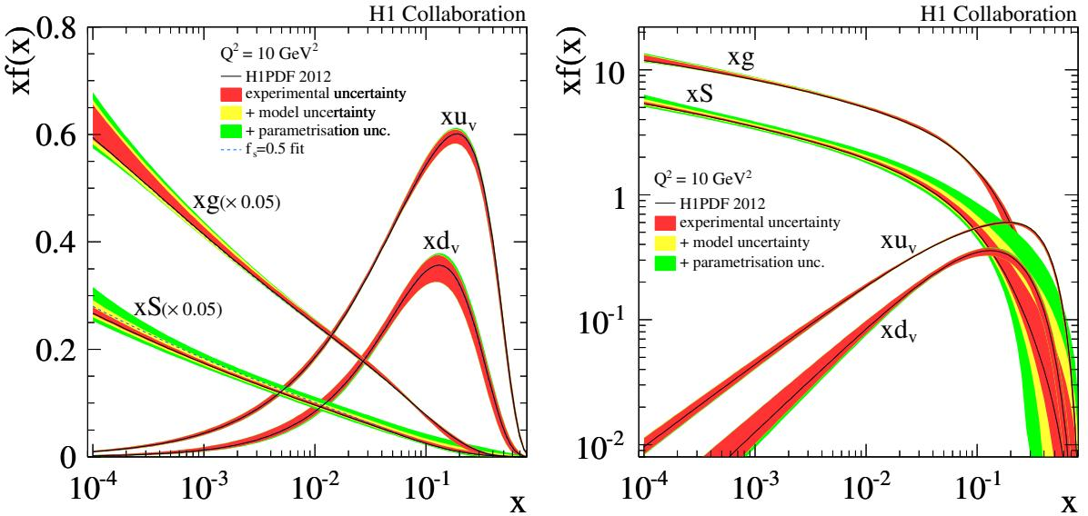
Figure 18: Parton distribution functions of H1PDF 2012 at the evolved scale of  $10 \text{ GeV}^2$ . The gluon and sea distributions in the linear scale plot (left) are scaled by a factor 0.05. The PDFs with  $f_s = 0.5$  are also shown. The uncertainties include the experimental uncertainties (inner), the model uncertainties (middle) and the parametrisation variation (outer). All uncertainties are added in quadrature.
