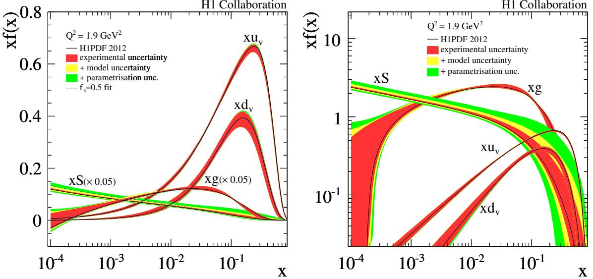
Figure 17: Parton distribution functions of H1PDF 2012 at the starting scale  $Q^2 = 1.9 \text{ GeV}^2$ . The gluon and sea distributions in the linear scale plot (left) are scaled by a factor 0.05. The PDFs with  $f_s = 0.5$  are also shown. The uncertainties include the experimental uncertainties (inner), the model uncertainties (middle) and the parametrisation variation (outer). All uncertainties are added in quadrature.
