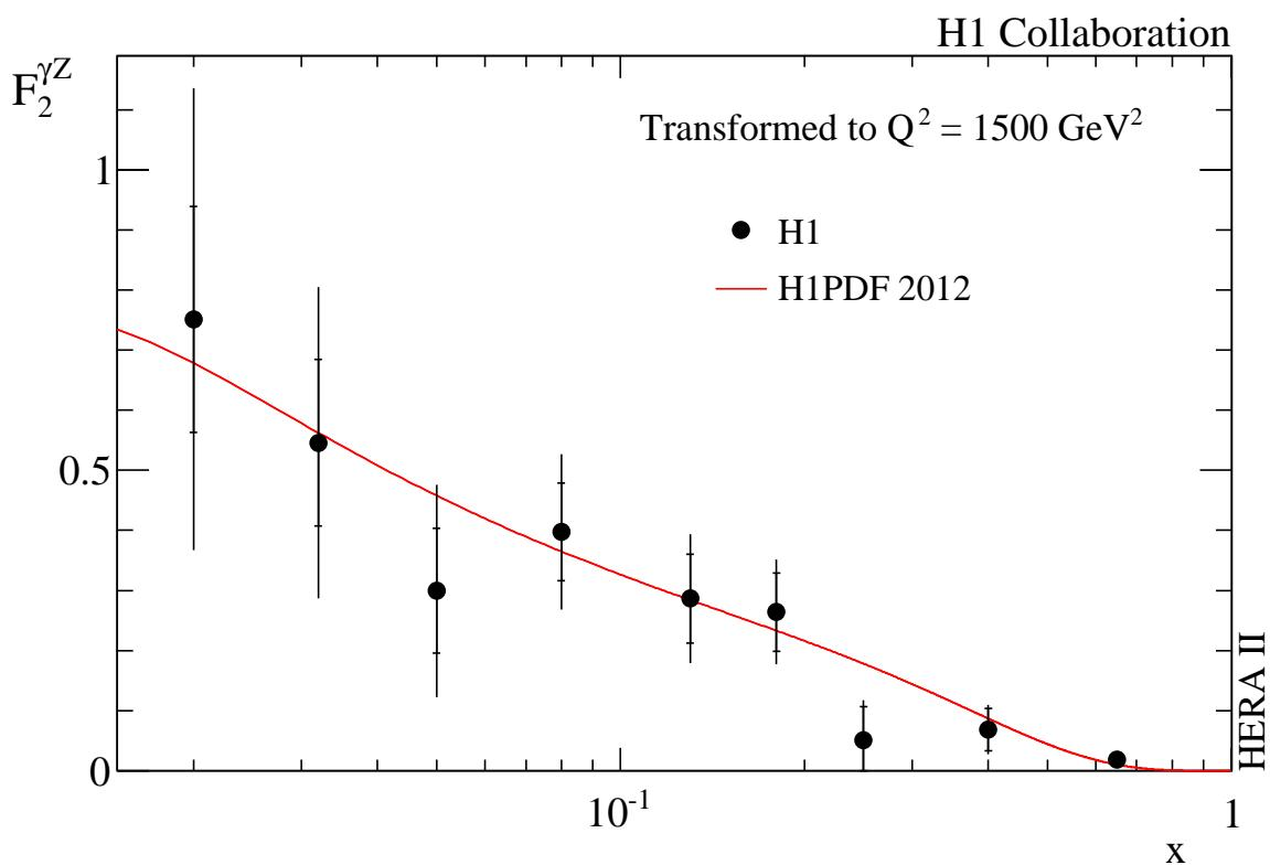
Figure 26: Structure function  $F_2^{\gamma Z}$  transformed to  $Q^2 = 1500 \text{ GeV}^2$  for data (solid points) and the expectation from H1PDF 2012 (solid curve). The inner error bars represent the statistical uncertainties and the full error bar corresponds to the total measurement uncertainty.
