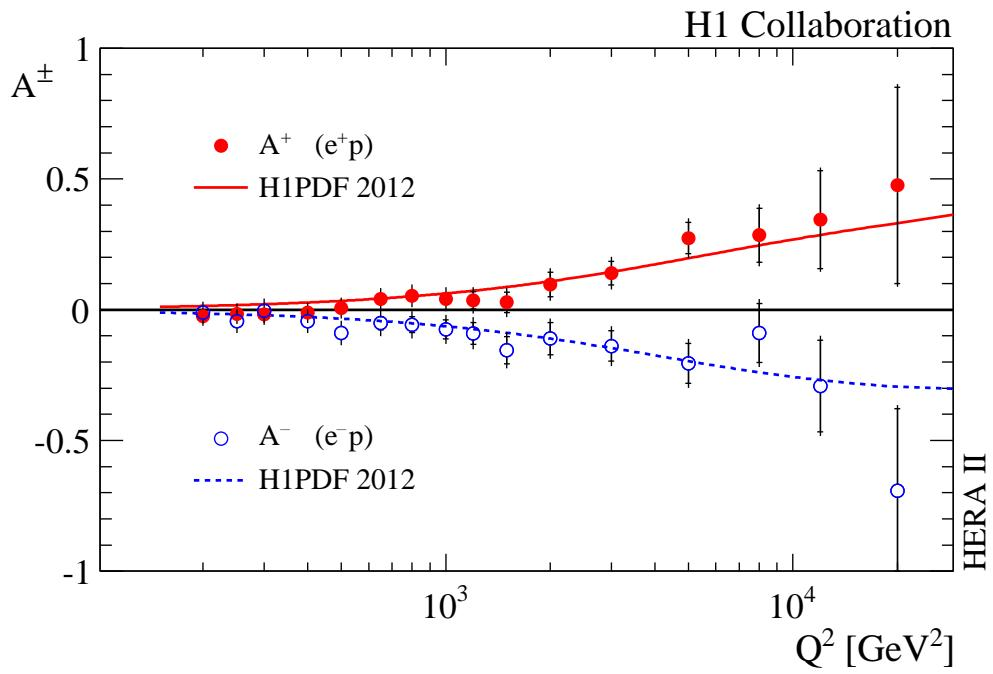
Figure 24:  $Q^2$  dependence of the polarisation asymmetry  $A^\pm$ , for  $e^+p$  (solid points) and  $e^-p$  (open circles). The data are compared to the Standard Model expectation. The inner error bars represent the statistical uncertainties and the outer error bars represent the total errors. The normalisation uncertainty is not included in the error bars.
