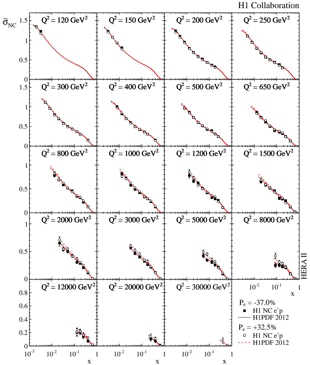
Figure 9: NC reduced cross sections  $\tilde{\sigma}_{NC}$  for  $e^+p$  L (solid squares) and R (open circles) data sets shown for various fixed  $Q^2$  as a function of  $x$ . The inner and outer error bars represent the statistical and total errors, respectively. The luminosity and polarisation uncertainties are not included in the error bars. The curves show the corresponding expectations from H1PDF 2012.
