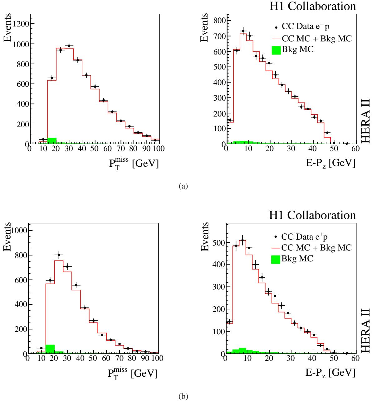
Figure 7: Distributions of  $P_T^{\text{miss}}$  and  $E - P_z$  for (a)  $e^-p$  and (b)  $e^+p$  CC data (solid points) and simulation (histograms). The estimated background contribution is shown as the shaded histograms.
