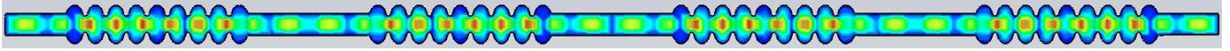
Figure 4.15: The electric field distribution of strongest coupled cavity mode from the first dipole band (frequency: 4.8076 GHz, R/Q : 125.762 \Omega/\text{cm}^2 per module). Electric (EE) boundary conditions were used in the simulation.
