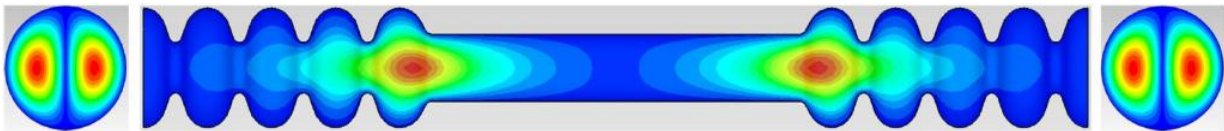
Figure 4.13: The electric field distribution of one dipole beam-pipe mode (frequency: 4.1481 GHz, R/Q : 1.544 \Omega/\text{cm}^2 ). Electric (EE) boundary conditions were used in the simulation.
