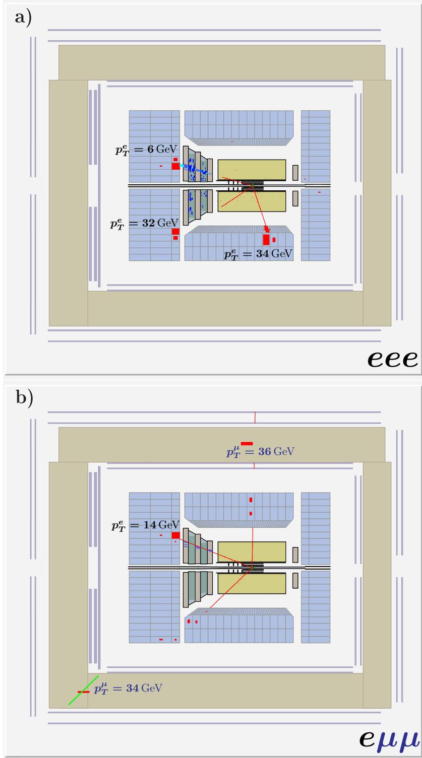
**Figure 1:** a) An event with three electron candidates in the ZEUS detector. The invariant mass of the two highest- $p_T$  electrons is  $M_{12} = 113 \text{ GeV}$ ; the corresponding transverse momenta are given above. b) An event with two muons and an electron candidate in the ZEUS detector. The invariant mass of the di-muon pair is  $77.5 \text{ GeV}$ ; the corresponding transverse momenta are given above.
