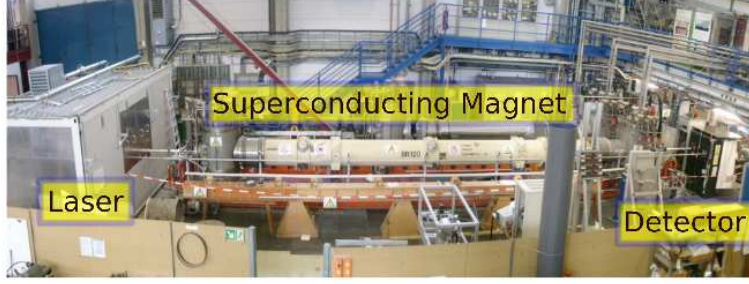
Figure 3. Schematic of a LSW setup (ALPS experiment at DESY). The laser is injected in the bore of the superconducting dipole magnet. An opaque wall is placed at the center of the magnet. WISPs produced in this part, called production side pass through the wall, to the regeneration side where can reconvert into light and continue to the detector in the end part of the experiment. Figure from reference [38].
