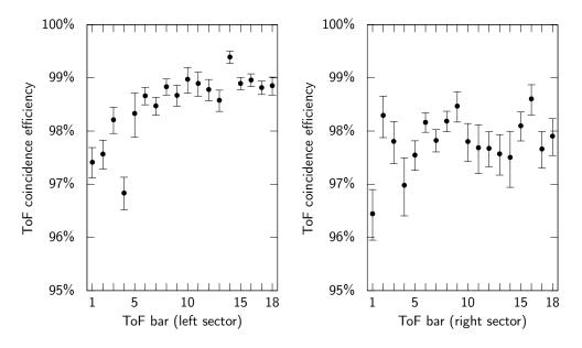
Fig. 16: Efficiencies for each TOF scintillator bar determined during the cosmic running period.
