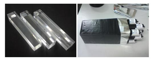
Fig. 24: Several of the  $PbF_2$  crystals used in symmetric Møller/Bhabha luminosity monitor before (left) and after (right) assembly with the PMT readout system.
