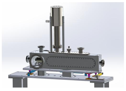
Fig. 4: CAD model of the OLYMPUS scattering chamber.
