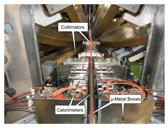
Fig. 23: A photograph showing the main components of the SYMB detector. The thick red line indicates the direction of the beam while the thinner red lines indicate the general path of scattered electrons, positrons, or photons entering the SYMB.
