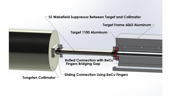
Fig. 6: CAD model of the wakefield suppressor between the collimator and the target cell.
