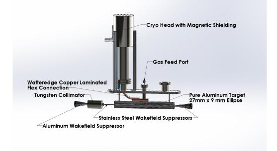
Fig. 5: CAD model of the target cell, wakefield suppressors, and collimator inside the OLYMPUS scattering chamber.
