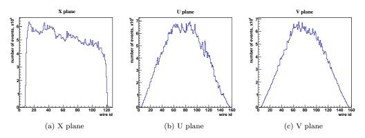
Fig. 21: Hit distributions for the X, U, and V planes of a single, representative MWPC detector. The distribution of events is determined by the detector acceptance and sense wire angle for each plane.
