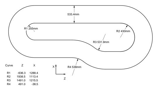
Fig. 10: Planar view of BLAST coil outline showing dimensions and position relative to the center of the target cell.
