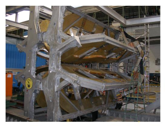
Fig. 9: The toroid magnet assembled at DESY before the subdetectors were installed
