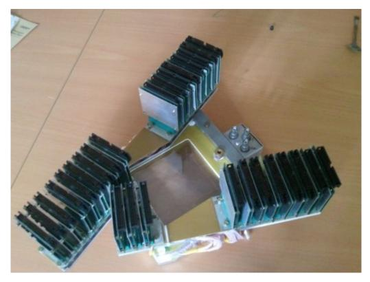
Fig. 20: Photograph of one MWPC with CROS3 readout electronics.
