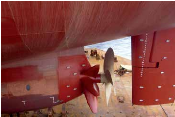
Figure 2: Photo taken in the dry dock just after the installation of PSS
