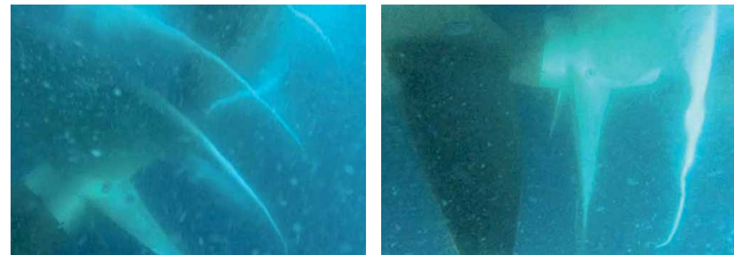
Figure 10: Propeller cavitation and cavitating hub vortex for ship without PSS (left) and propeller cavitation for ship with PSS (right)
