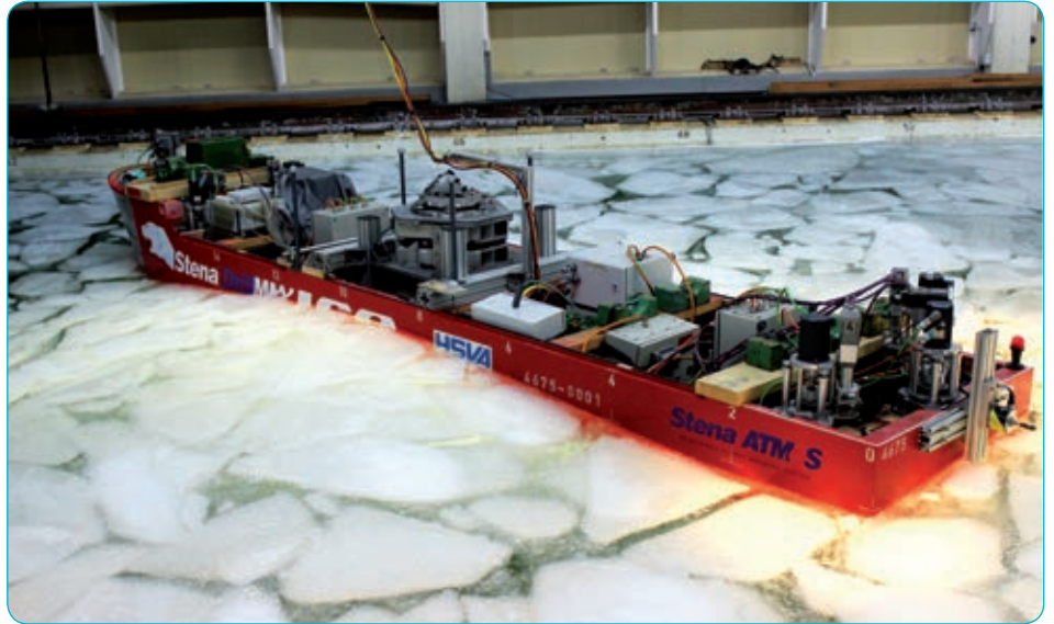
Fig. 7: Floating structure in ice covered waves of 0.1 m wave height
