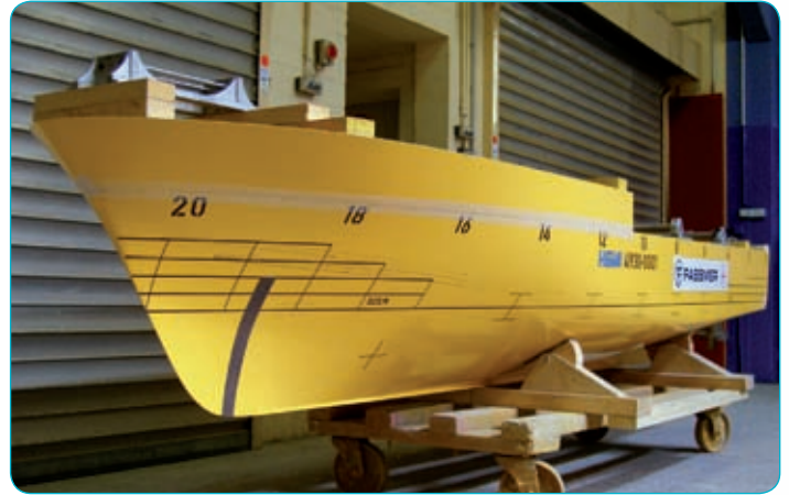
Fig. 3: The 1/6 scaled model for the powering tests
