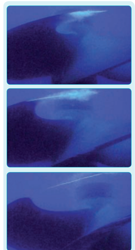
Fig. 2: Cavitation on a 9 m diameter container ship propeller at 70 RPM, taken by the miniature camera just through a 20 mm bore in the shell plating
