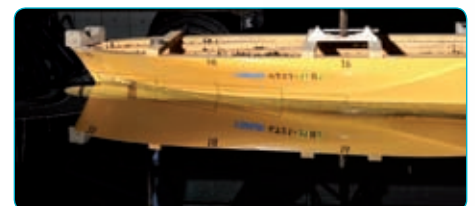
Photo 4: Full load draught and high speed – ES-Bow
