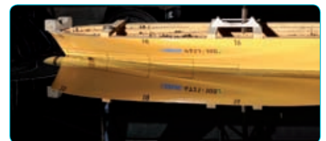
Photo 3: Full load draught and high speed – conventional bow
